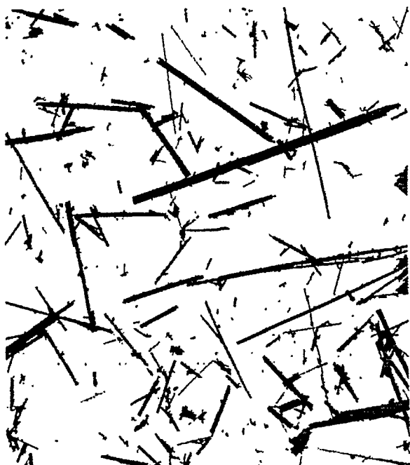
FIG. 2.—Electronmicrograph of UIC crocidolite ( \times 1875 ).
