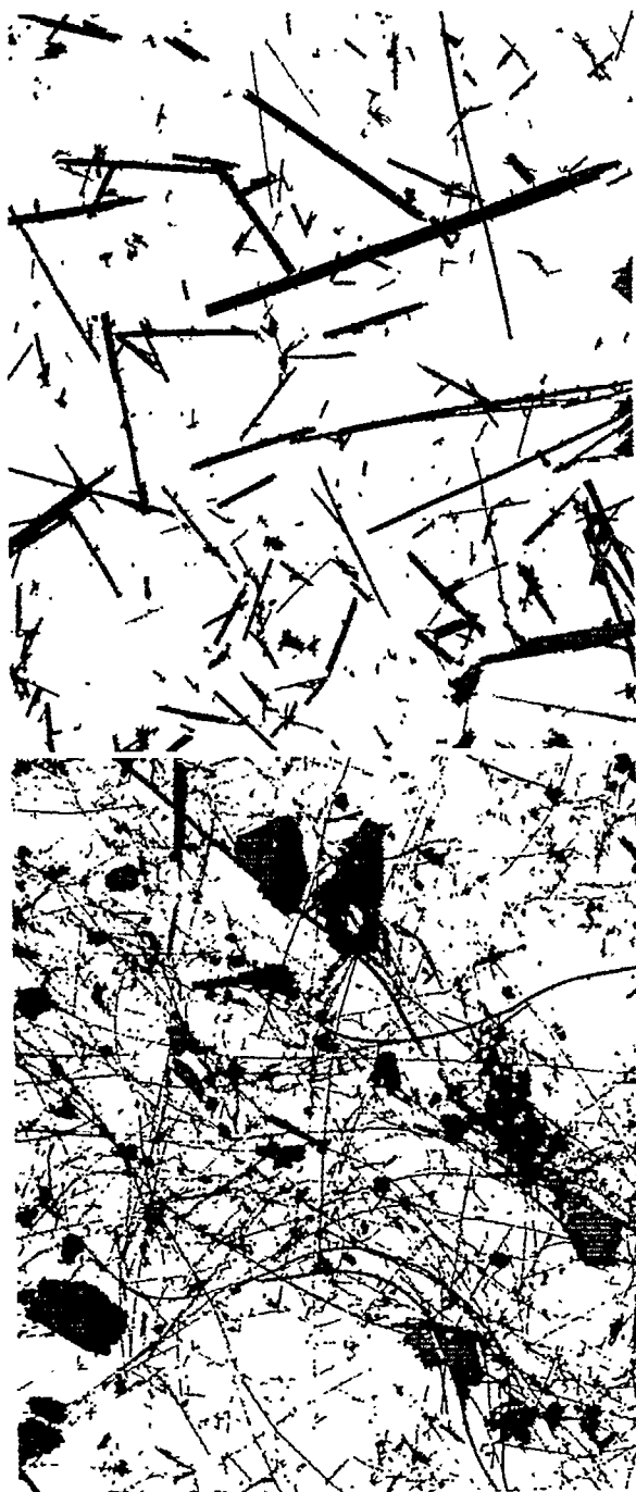
FIG. 2.—Electronmicrograph of UIC crocidolite ( \times 1875 ).
