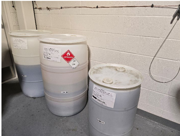
Photo I: CAA – Hazardous waste (toluene and methanol), non-hazardous waste, and used oil containers
