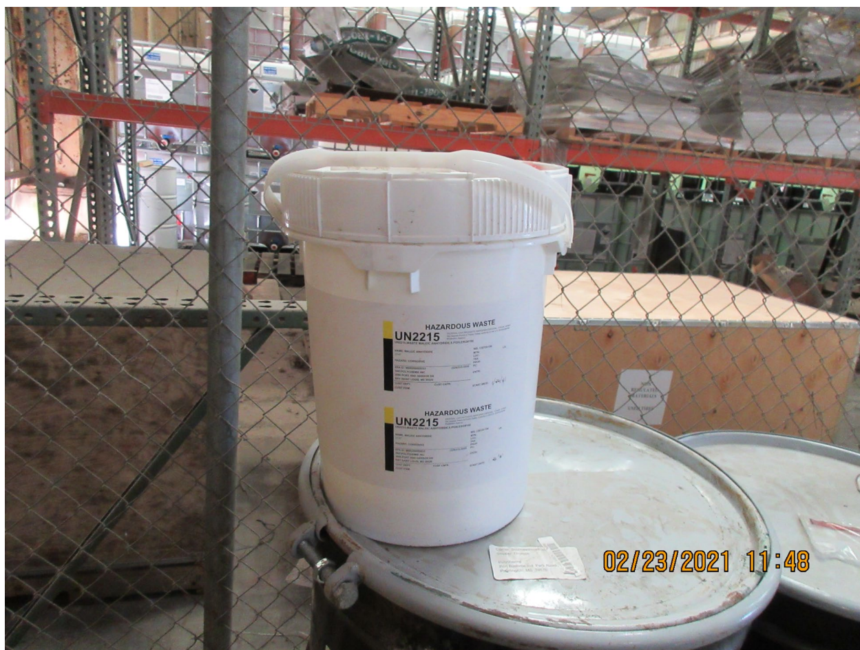
Photo 5 – 5-gallon container of hazardous waste within 90-day accumulation area missing an indication of the hazard within the container.
