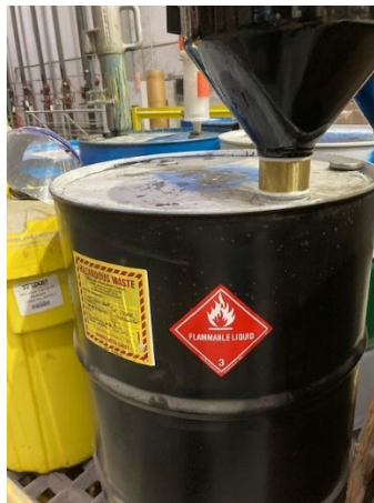
Photo-2 Main Accumulation Point, 1 55-gallon SAA container marked with hazard indication
