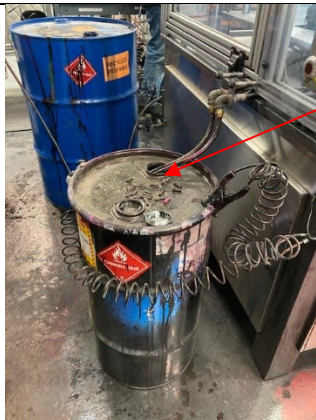
Photo-3 Sharpie Fine #13, 1 30-gallon SAA open container containing flammable spent solvent waste
