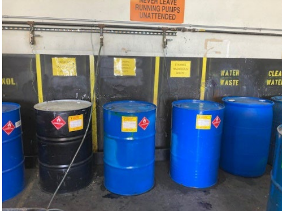
Photo-7 Ink Consolidation Room, 3-containers received solvent waste for consolidation from Satellite areas in the production area. The containers shall be managed as 90-day containers and require an accumulation start dates on all the three containers
