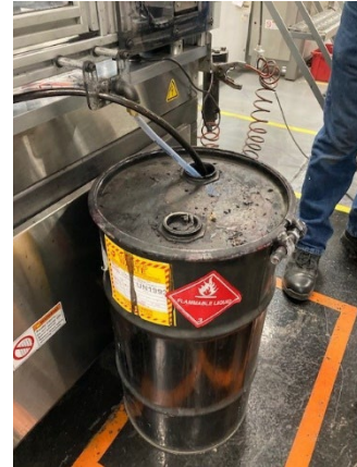
Photo-4 Expo Marker Line #11, 1 30-gallon SAA open container containing flammable spent solvent waste
