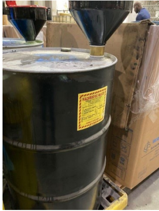
Photo-1 Main Accumulation Point, Failure to provide hazard indication on 1 55-gallon SAA container of inkjet cartridge
