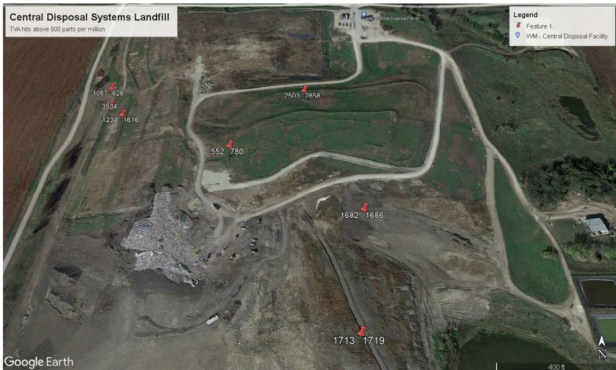
Figure 1. Areas surveyed with the Toxic Vapor Analyzer with respective methane values over 500 parts per million (ppm)
