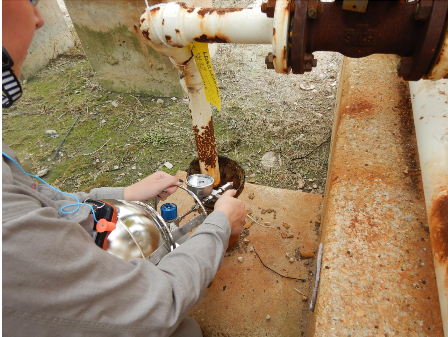
Photo 1165: Summa cannister collection of F-220 seal pot drain - 5/4/23 10:01 DSCN1165.jpg
