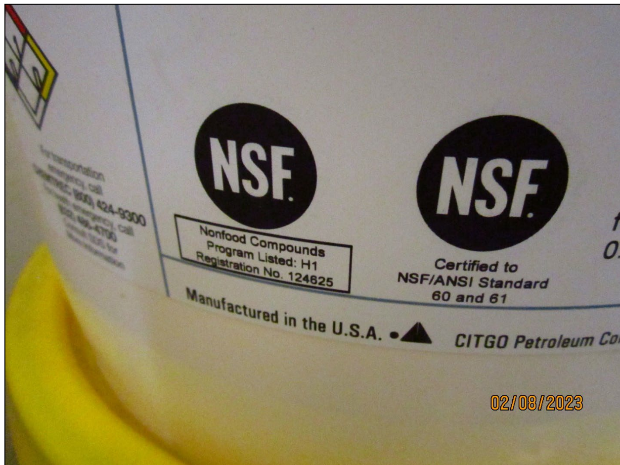
Photograph 39. Food Grade Lubricant, Treatment Room Close up view of the Clarion food grade machinery lubricant label that was being stored in the treatment room. The lubricant was NSF/ANSI 60 and 61 standard certified.
