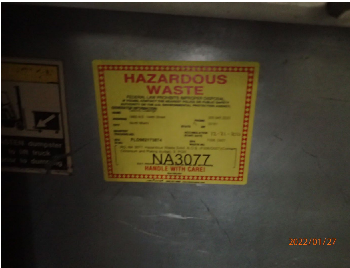
Photo 5: The metal container box under the sludge dryer was labeled “Hazardous Waste—Chromium Plating Sludge” and dated 12/21/2021. The container also had a Class 9 D.O.T. placard which represents “miscellaneous good” and does not specify the specific hazards.
