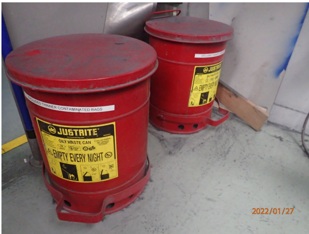
Photo 1: Two (2) 6-gallon closed containers for excluded solvent-contaminated rags, closed, and labeled. The containers were not dated to demonstrate that the excluded solvent-contaminated rags were not exceeding the 180-day accumulation time limit.
