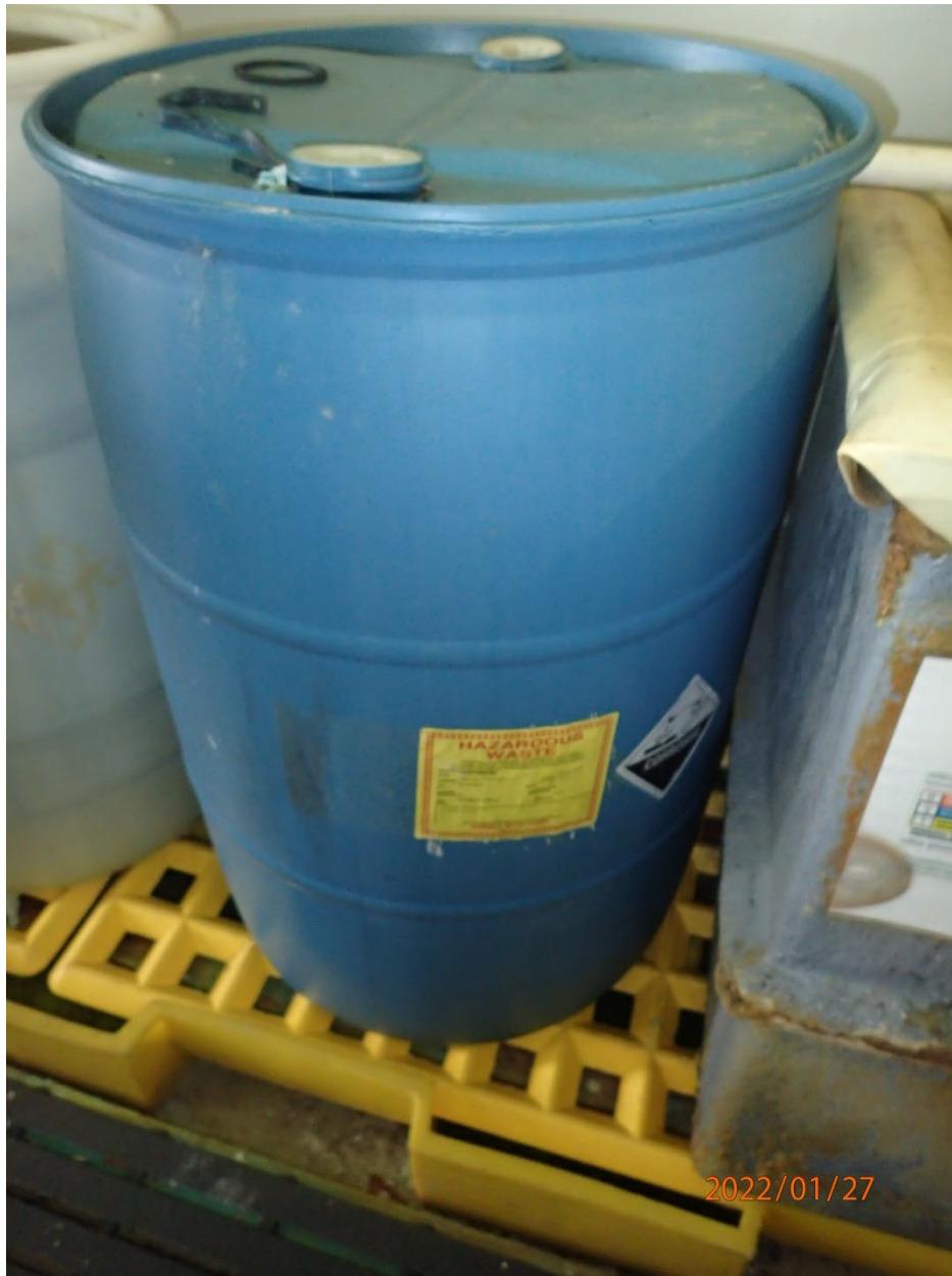
Photo 17: One (1) 55-gallon closed drum of sulfuric acid, labeled “Hazardous Waste”, and marked with an indication of hazard
