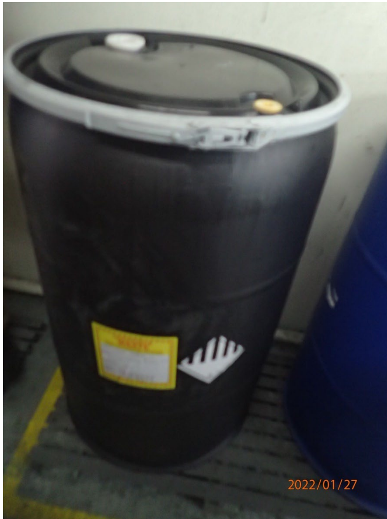
Photo 8: Wastewater treatment sludge with a hazardous waste label that contained the accumulation start date and marked for Toxic. CAA1.
