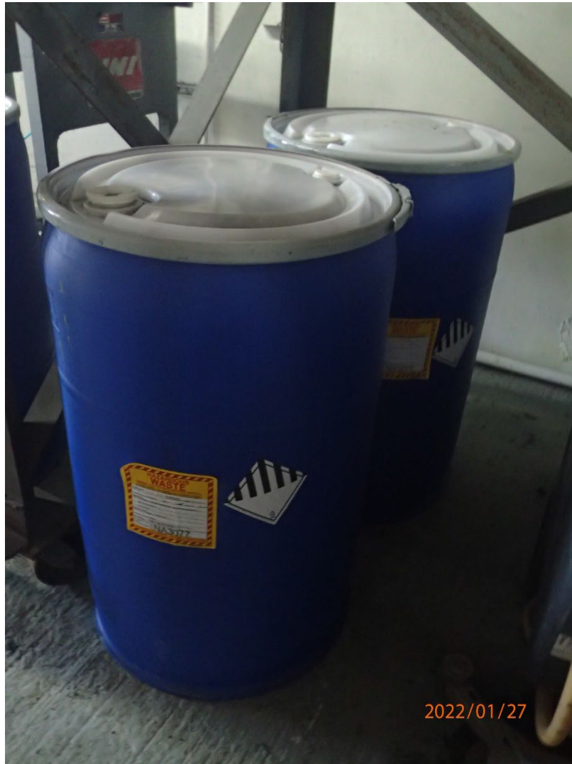
Photo 6: Wastewater treatment sludge with a hazardous waste label that contained the accumulation start date and marked for Toxic. CAA1.
