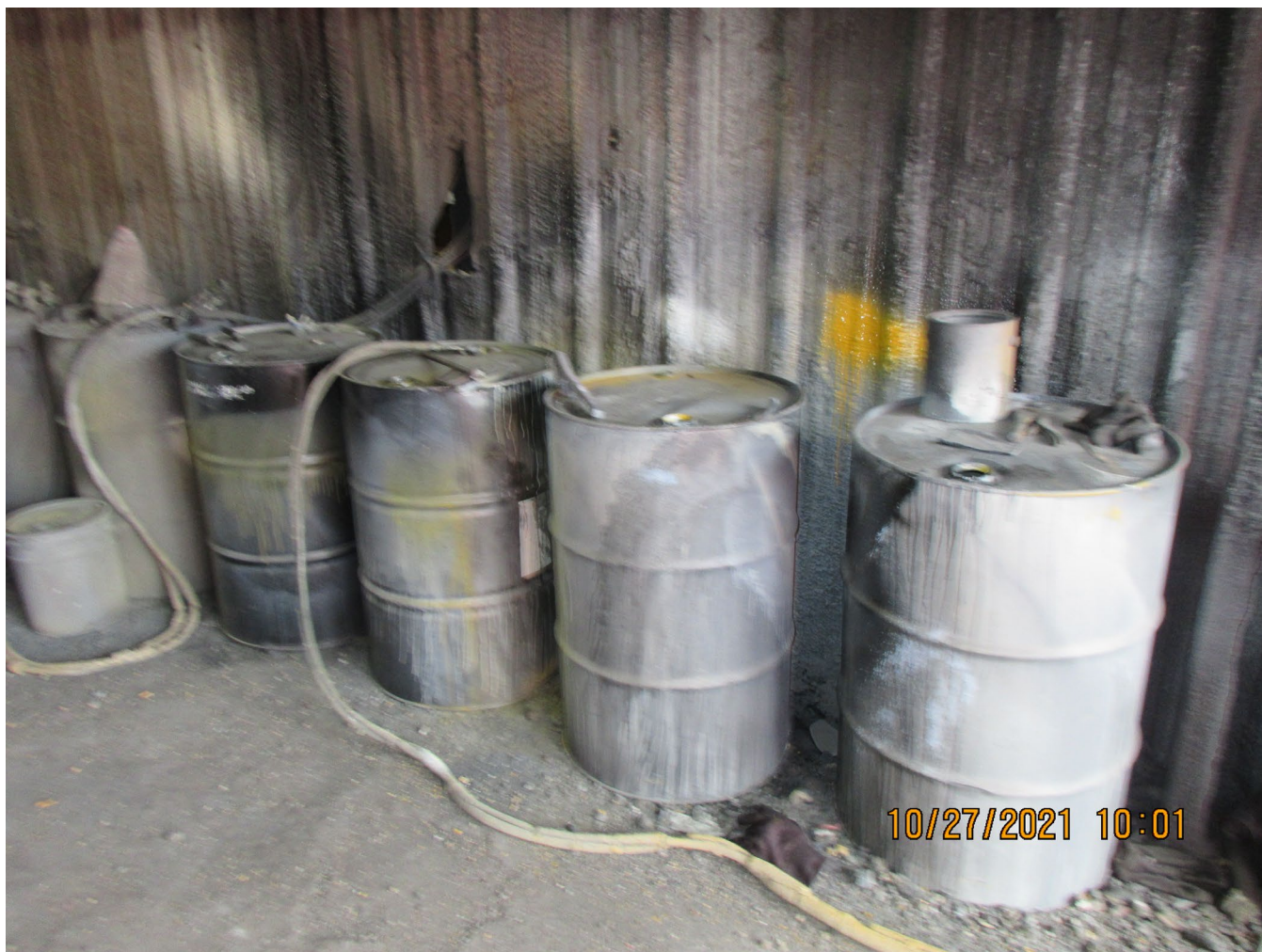
Photo 1 – Four drums accumulating spent acetone in SAA within Paint Room
