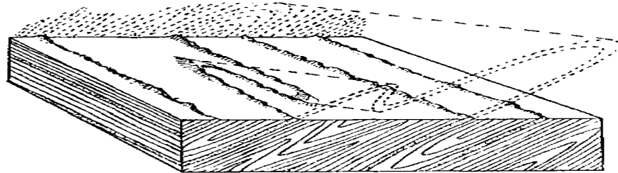
Figure 12 Section and sketch of pitching isoclinal fold to illustrate the manner in which pitch carries a bed below ground; the line of outcrop of the ridge of resistant rock formed on the left flank of the main anticline is very similar to the margin of the garnet-gneiss tongue as shown on the sketch in figure 9.
