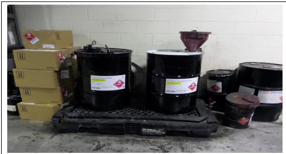
Hyundai. Paint Mix Room - Solvent Side. Inspectors observed two 55-gallon containers accumulating waste paint and solvent and solvent-borne waste from mixing paints and solvents. The containers were marked with dates in June and July 2021. Photograph 7 taken July 26, 2021 at 3:20 p.m.
