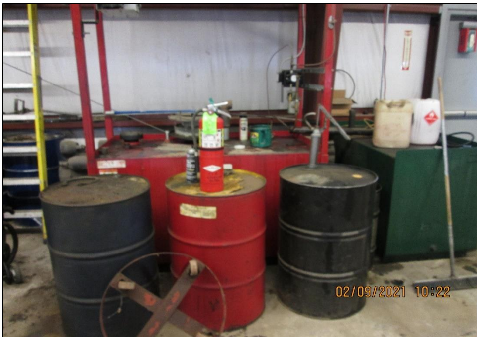
Photograph 10. View of three 55-gallon drums containing used oil inside of the “American Building.” All containers were inside of a covered building, but lacked secondary containment.
