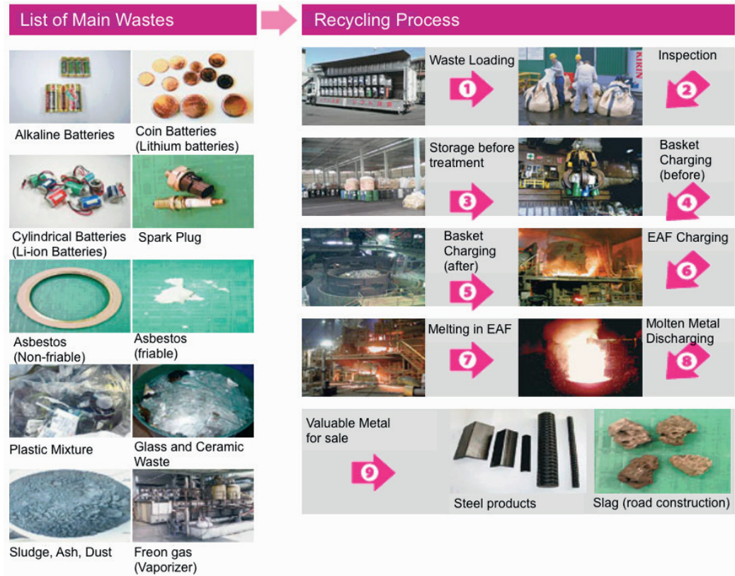
Figure 10: Flow chart of waste (including Li-ion batteries) recycling process published by Kyoei Seiko [26]
