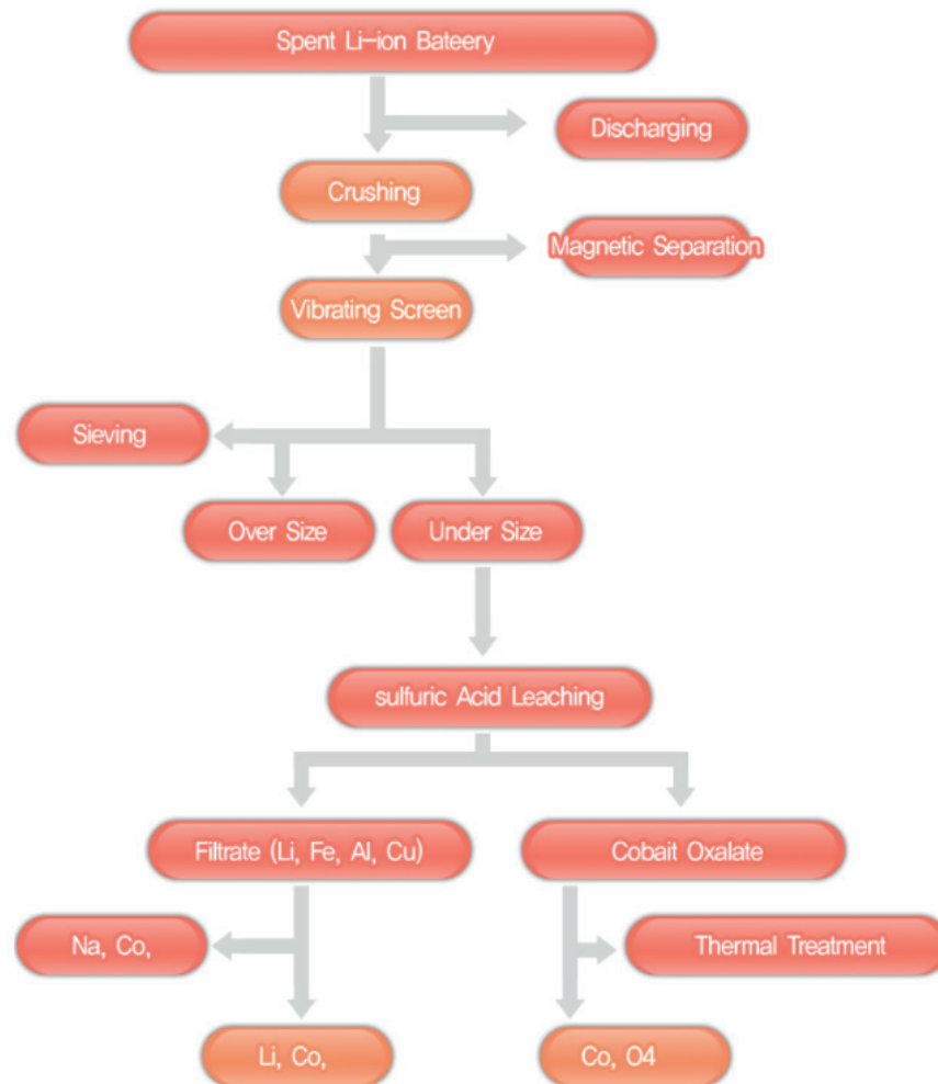
Figure 14: Flowchart of Li-ion battery recycling process published by Kobar [67]
