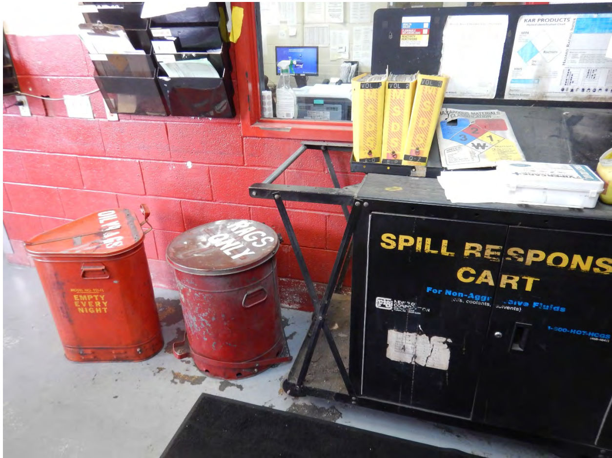
# 273 – Spill response area with rag containment
