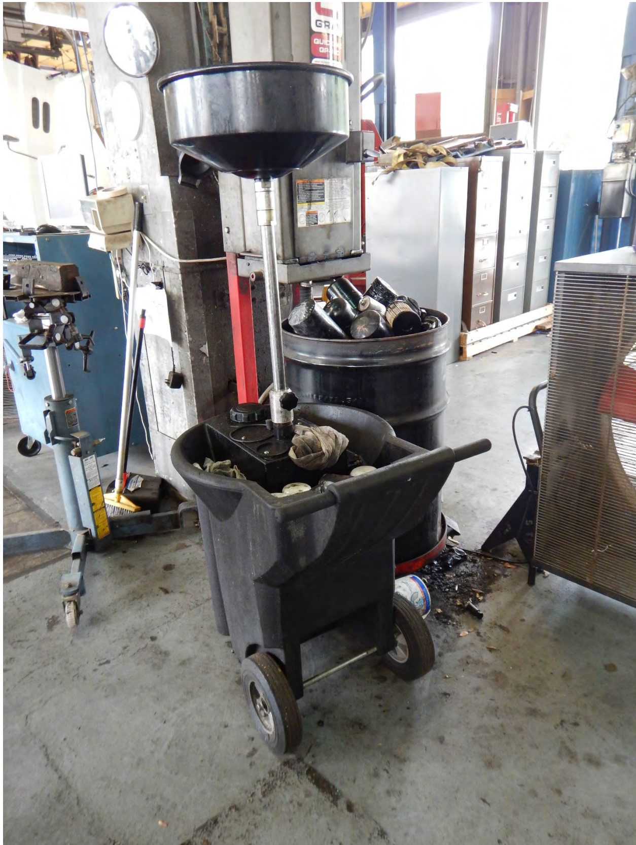
# 222 – Filter Recycling / used oil receptacle #1
