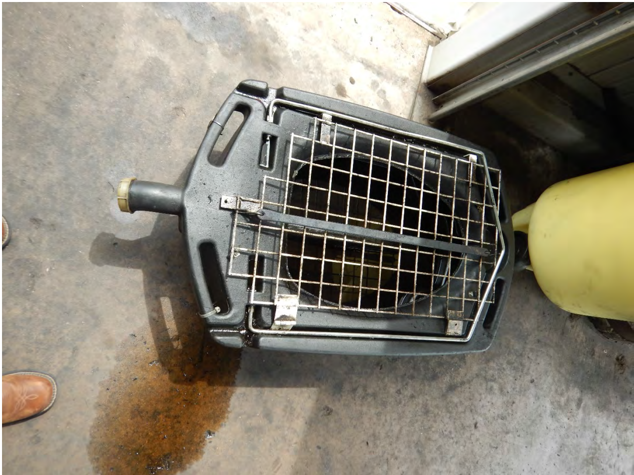
# 266 – Unattended Spill From Oil Collection Container
