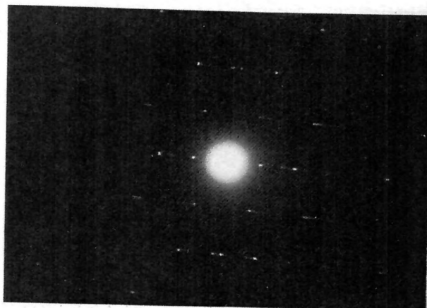
Figure 3 Selected area electron diffraction pattern for a single chrysotile fiber.
