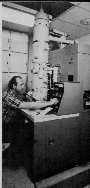
Figure 1 Model 200KV transmission electron microscope.
