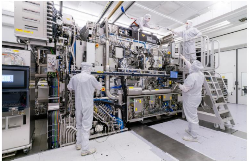
Figure 10-1 ASML Latest Extreme Ultraviolet Photolithography Exposure Tool. 79
