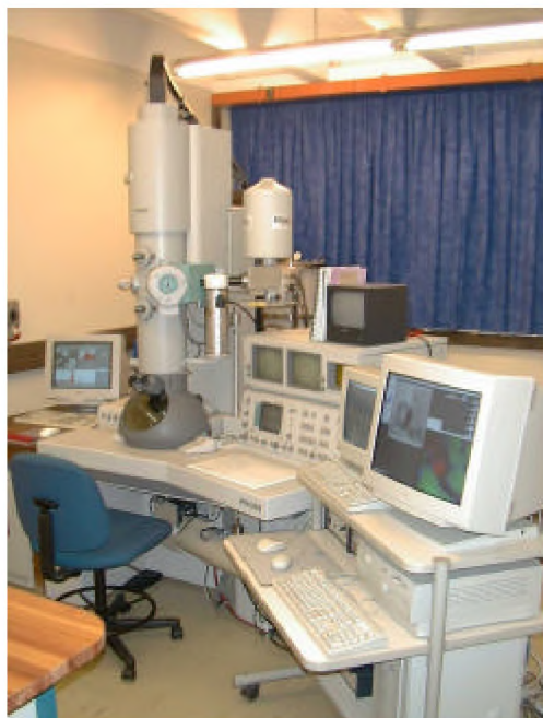
Figure 2.2: The transmission electron microscope that was used in the study.
