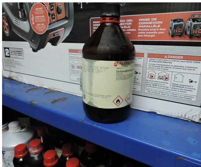
Picture 26 - UPR CIVIL ENGINEERING- At the Lab CI 018 Blue Cabinet Flammable there were two (2) 4-L bottles containing Dichloroethane leaking and covered with moisture, dated January 22, 2011 which decomposes into carbon dioxide and in presence of heat it can produce toxic fumes such as methylene chloride.
