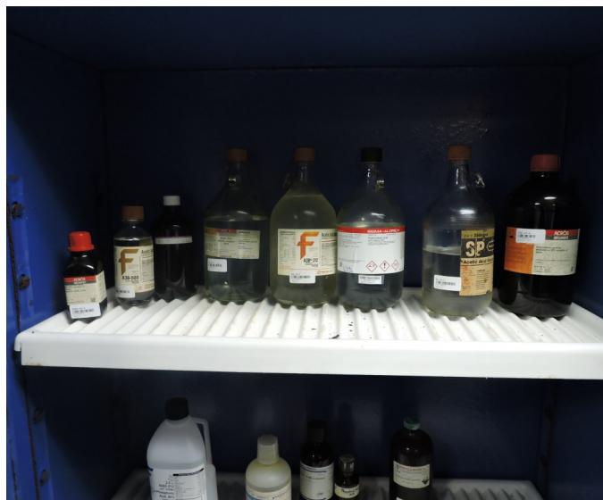
Picture 32 - UPR CIVIL ENGINEERING— At the Lab ICI 018 Blue Cabinet Corrosive there were three (3) 4-L ambar bottles containing Hydrochloric Acid, dated January 27, 2020, deteriorated conditions and labels being vanished. Acetic Anhydride is not compatible with Hydrochloric Acid and should not be stored
