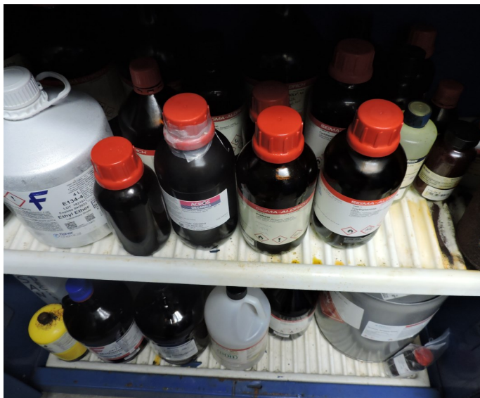
Picture 29 - UPR CIVIL ENGINEERING- At the Lab CI 018 Blue Cabinet Flammable there was one (1) 4-L ambar bottle containing Titanium Isopropoxide, dated August 2019, which is incompatible with strong oxidizing agents and strong acids
