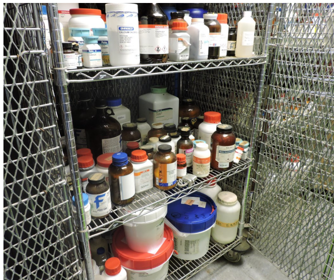
Picture 38 - UPR CIVIL ENGINEERING- At the Lab CI 018 EPA Inspectors observed numerous expired chemicals (since < 1986), discarded, contaminated, various unused chemical reagents, deteriorated and stored for a long time in shelves without physical protection each other from incompatibility characteristics.
