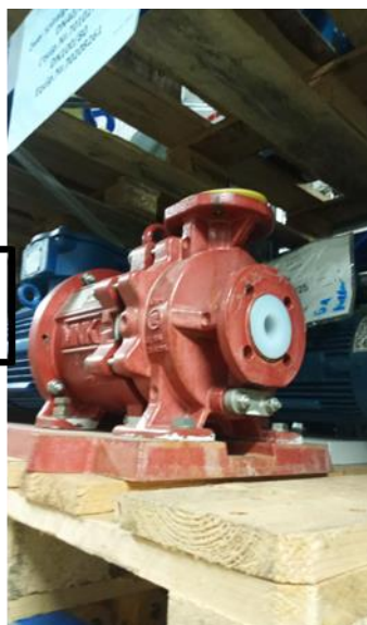
Pump with PTFE inliner
