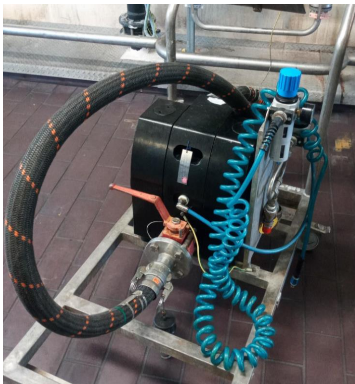
Picture 9 Mobile pump with body, hose, and sealings made of PTFE
