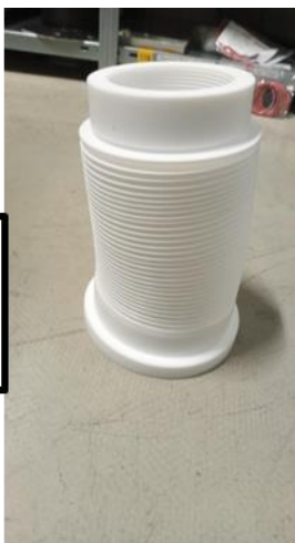
Corrugated bellow made of PTFE
