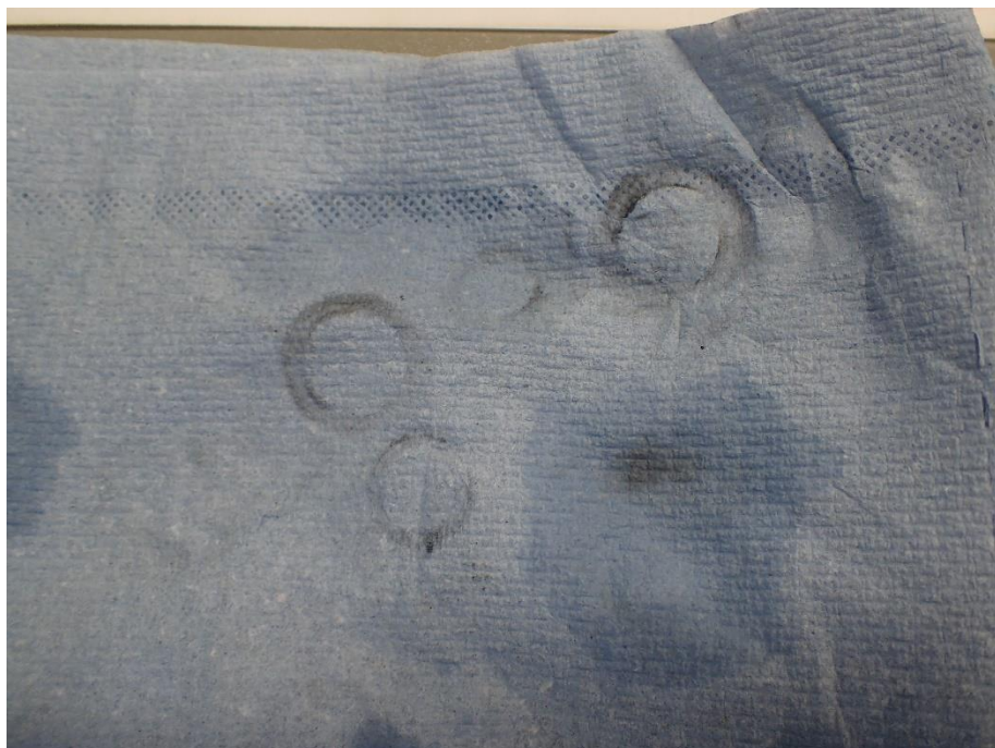
Picture 25 Coloration of paper towel used for drying of NBR component after 96h exposure to heptane
