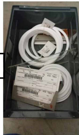
Gasket made of PTFE
