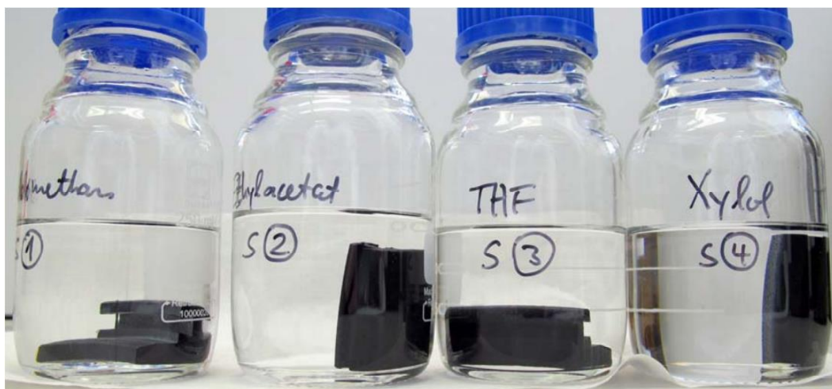
Picture 28 Sample bottle with black PTFE and different solvents after 40 d exposure at 80°C
