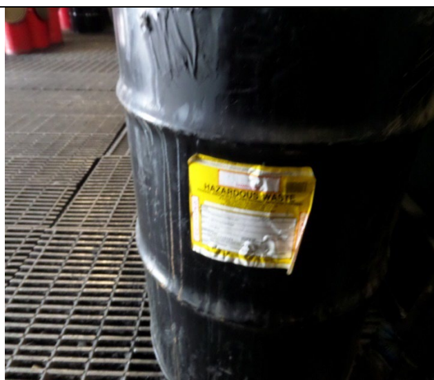
Branch Sales to Service. Container of waste solids debris missing flammable solids hazard indicator. Photograph 16 taken at 11:32 a.m.
