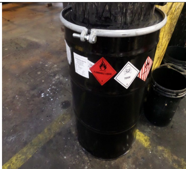
Antifreeze/Machine Return Area. SK representative labeled the container with all hazard indicators. Photograph 14 taken at 11:21 a.m.
