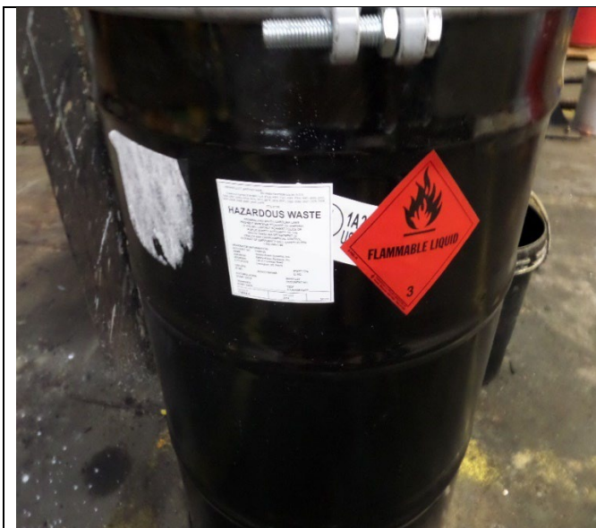
Antifreeze/Machine Return Area. The inspectors observed a 55-gallon container not labeled with all hazard indicators. Photograph 13 taken at 11:18 a.m.
