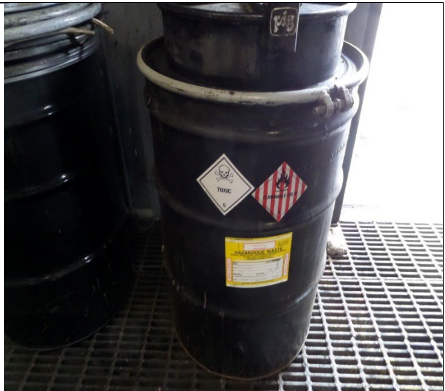
Branch Sales to Service. SK representative labeled the container of waste solvent sludge with larger hazard indicators. Photograph 20 taken at 11:45 a.m.
