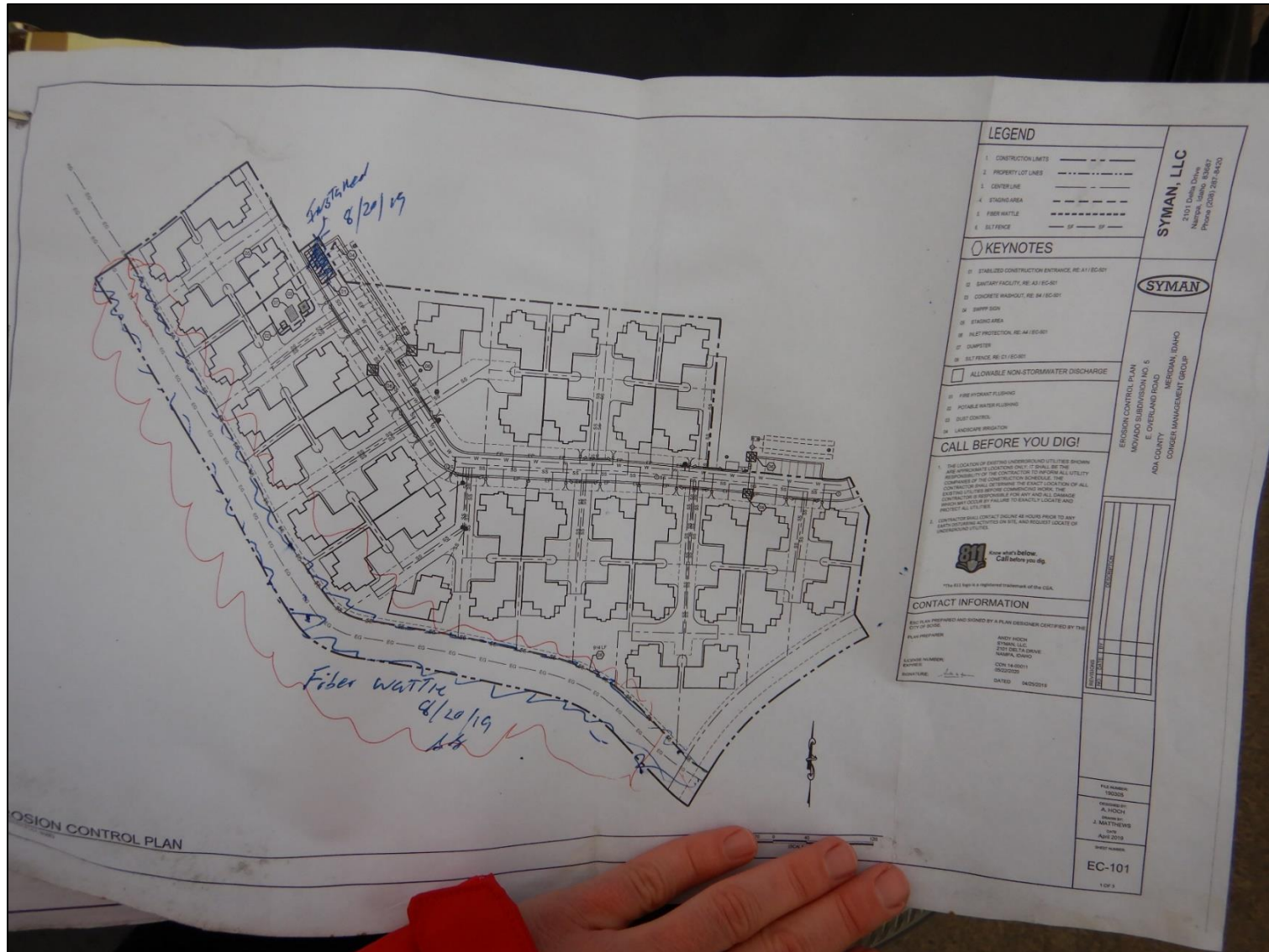
Exhibit 3. Image of the Site map of Phase 5 provided on Site of Movado Subdivision No. 5, 7, and 9. It was noted that the Site map does not identify all locations of stockpiles.
