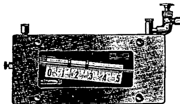
SINGLE-TUBE INCLINED: This gage is for small boilers and furnaces, and for power boilers with operating draft not over ¼ inch. It is equipped with seal for 250 feet chimney height.
