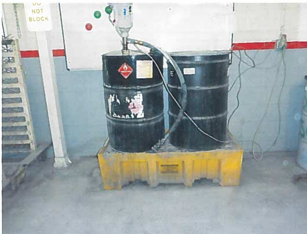
Photo 3: Two 55-gallon drums on portable secondary containment in the Shakespeare area. Although one drum is labeled as recycled acetone, the other is labeled as hazardous waste flammable liquid containing acetone and MEK. Mr. Senn stated that the drums have been reused, but that the labels were not removed. He stated that these drums both contain clean acetone for use on-site.
