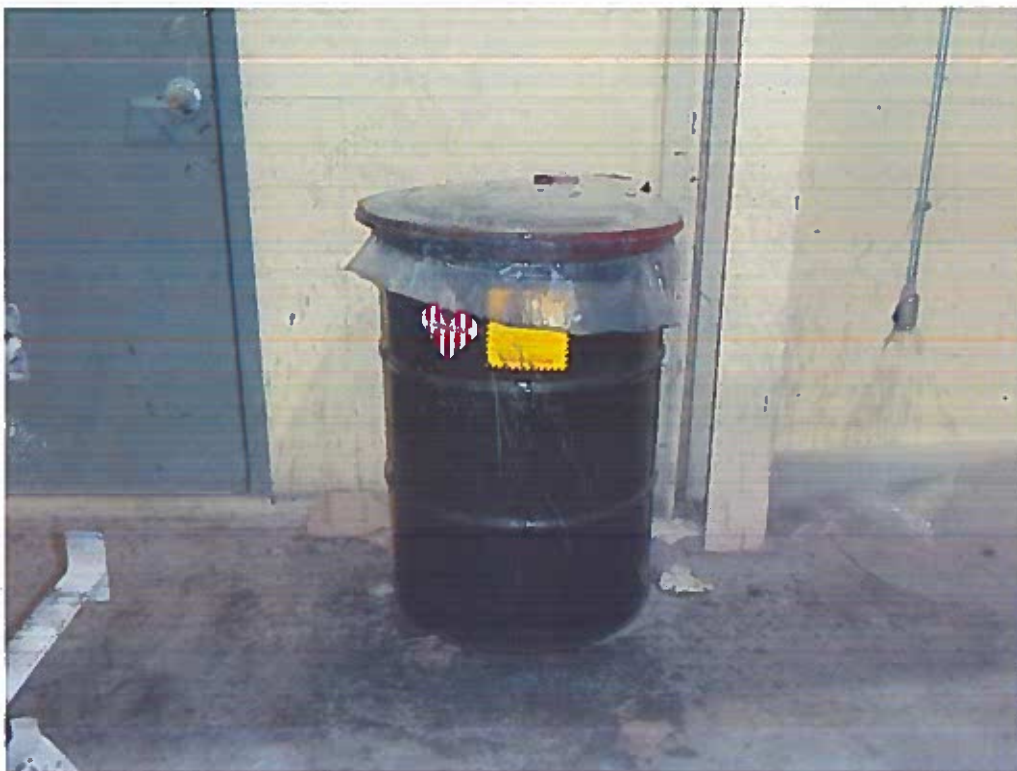
Photo 14: SAA for accumulating solvent contaminated rags used in the winding area within the Light Pole Building.
