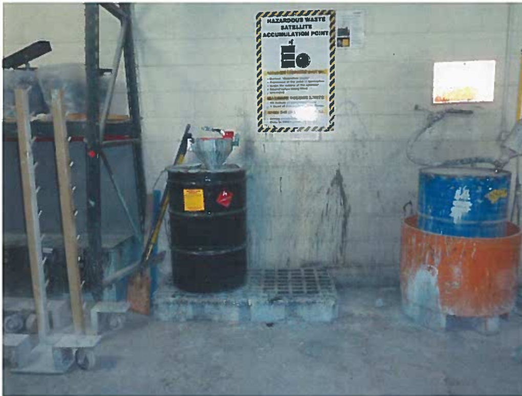
Photo 7: SAA for accumulating waste paint related material generated in the paint booth within the Main Building.
