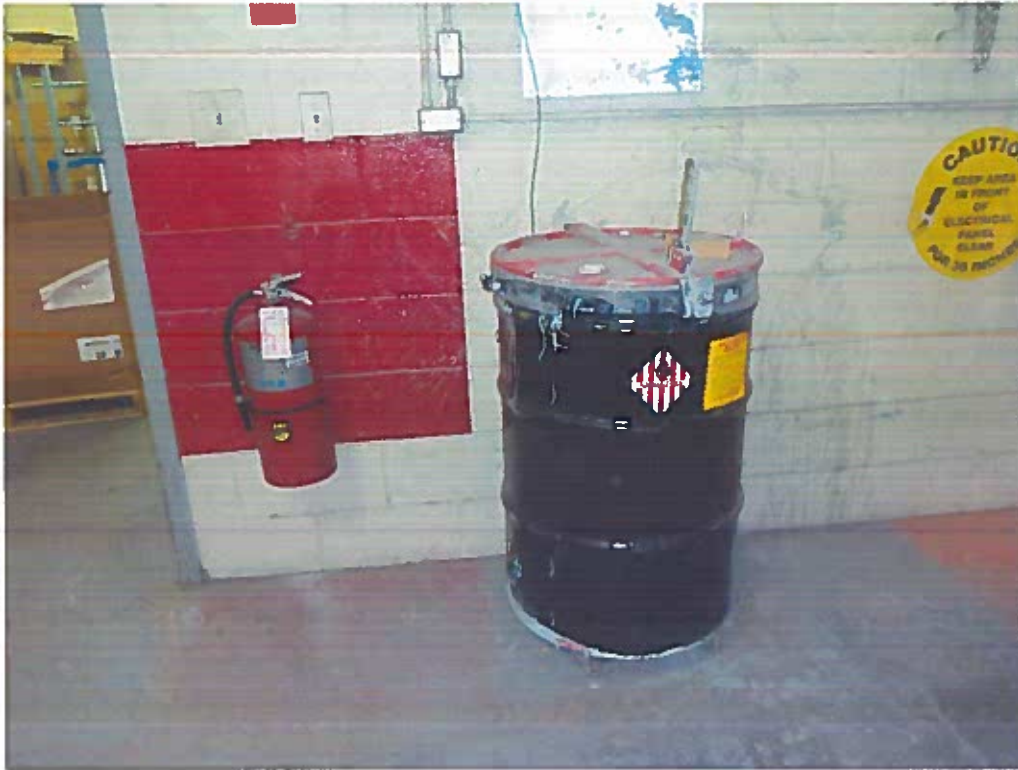
Photo 6: SAA for accumulating solvent contaminated rags used in the manual painting area within the Main Building.
