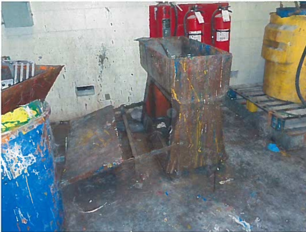
Photo 5: Old acetone parts washer used to clean parts removed from the protrusion lines in the Carsonite area.
