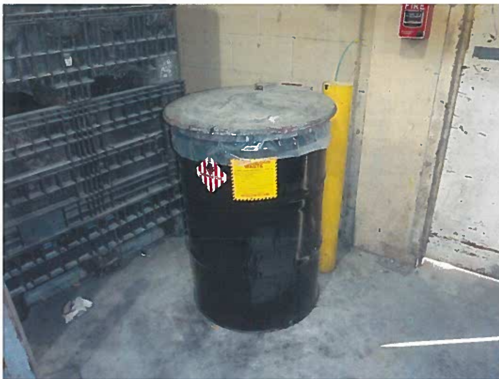
Photo 19: SAA for accumulating solvent contaminated rags generated in the manual painting booths within the Light Pole Building.
