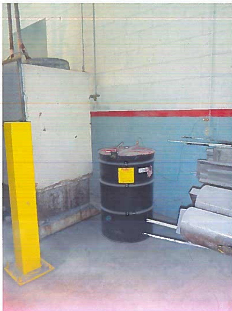
Photo 2: SAA for accumulating solvent contaminated rags used in cleaning protrusion machines in the Shakespeare area.
