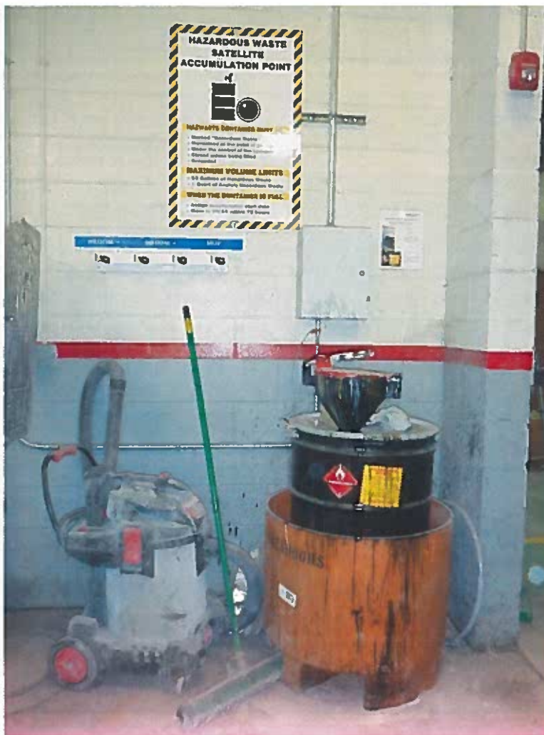
Photo 9: SAA for accumulating waste paint related material generated in the dip tank area.
