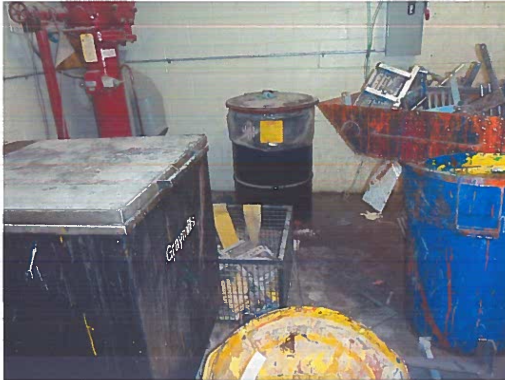
Photo 4: New parts washing unit (black box with gray lid) on the left, and SAA in the corner for accumulating solvent contaminated rags used in cleaning protrusion machines in the Carsonite area.
