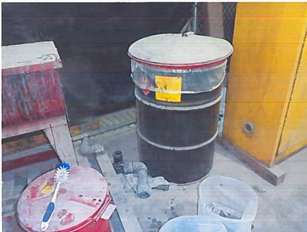
Photo 8: SAA in the Maintenance Area for accumulating used aerosol cans generated throughout the facility.
