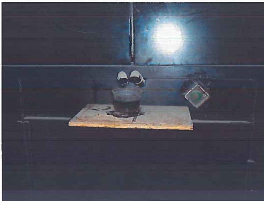
Photo 28: Point of generation for hazardous waste epoxy / glue at one of the on-site mixing stations.
