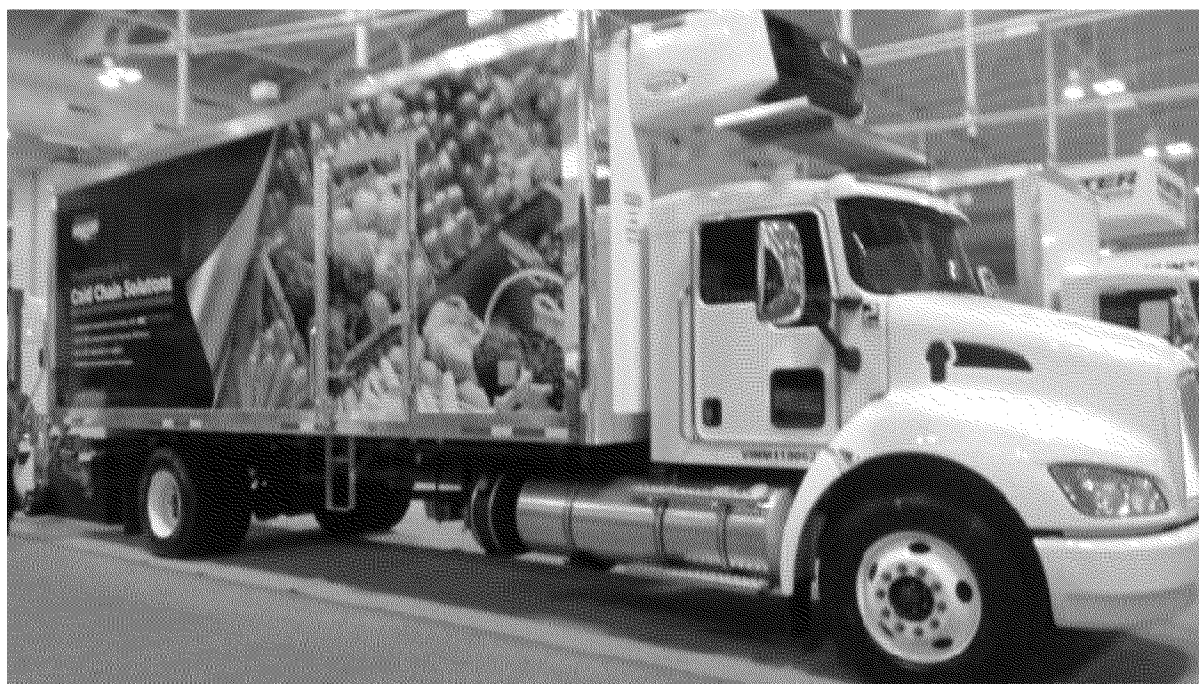
Figure 9. Refrigerated Truck Body- Wabash Prisma Construction
