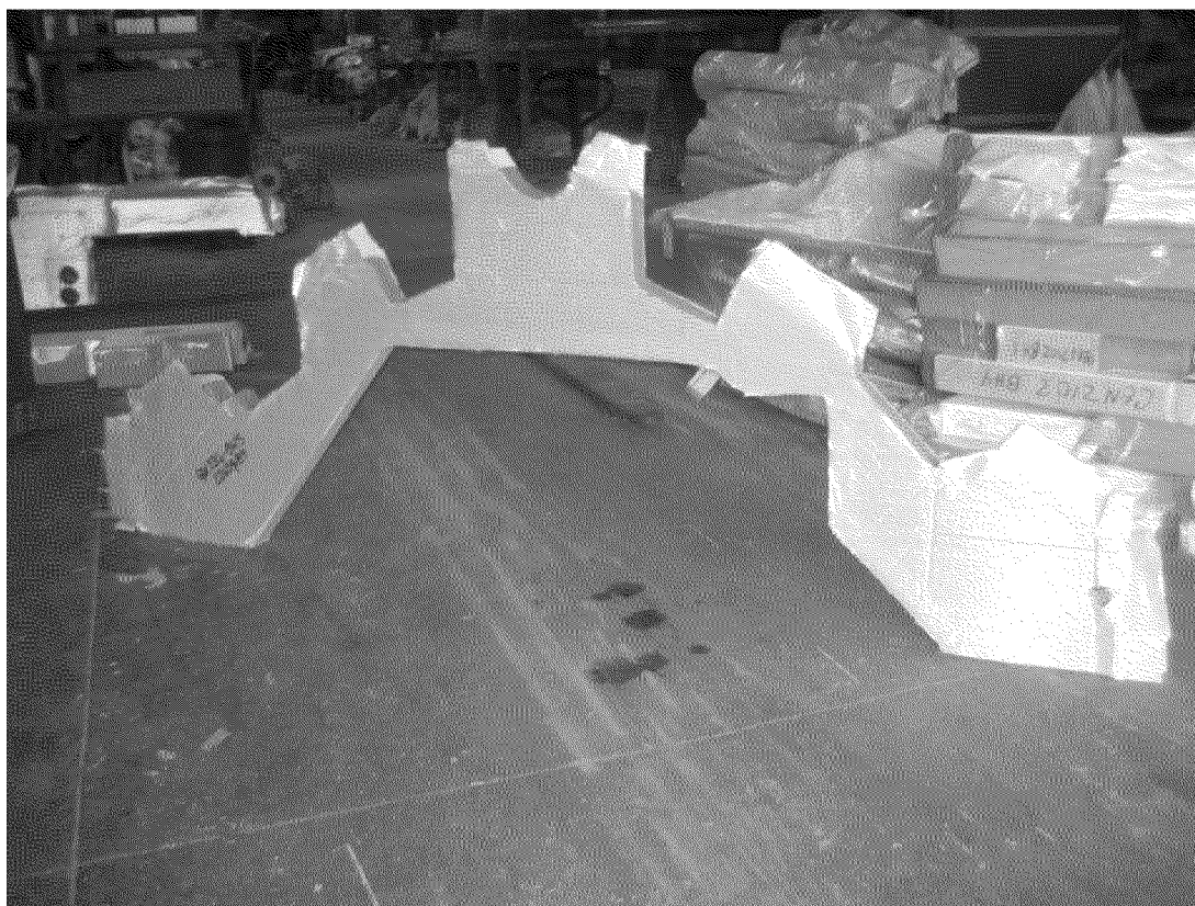
Figure 5. Large Bulkhead Prisma- Grady White 336. Component is shown before installation into the hull of the boat.
