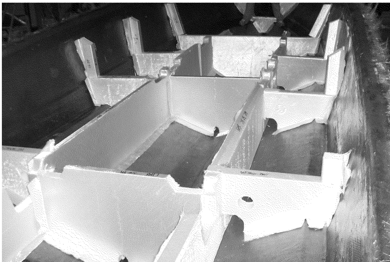
Figure 4., Large Boat Prisma System- Wellcraft. Again, the bulkhead and stringers shown are made of Prisma and replace wooden, fiberglass, or other materials.
