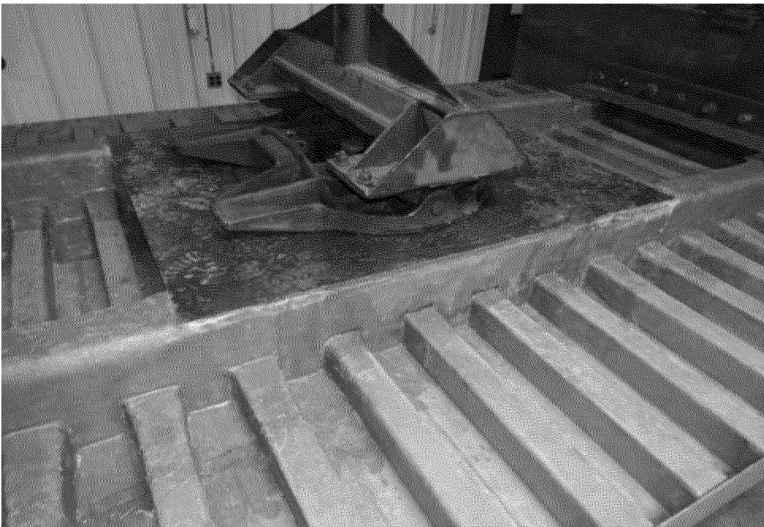
Figure 7. Coupler Plate Prisma Framed Floor- Qualification Testing at Wabash- Laminated Prisma Frames
