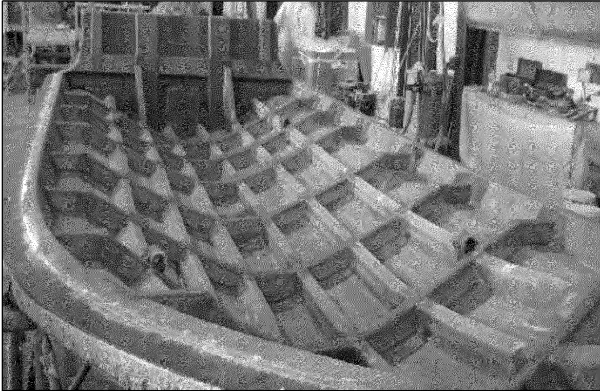
Figure 1. Advanced Design Lightweight Navy Combatant Craft Hull. All of the beams shown in this photo are made of Prisma. These beams replace traditional wooden or other composite framing in the hull.
