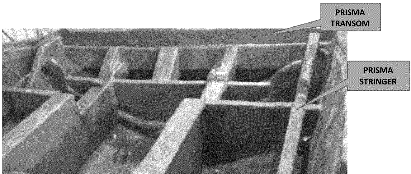
Figure 2. Transom and Aft Stringer Structure for the Hydrasports 53, the world's Largest Outboard Powered Center Console. These components are Prisma (shown laminated).
