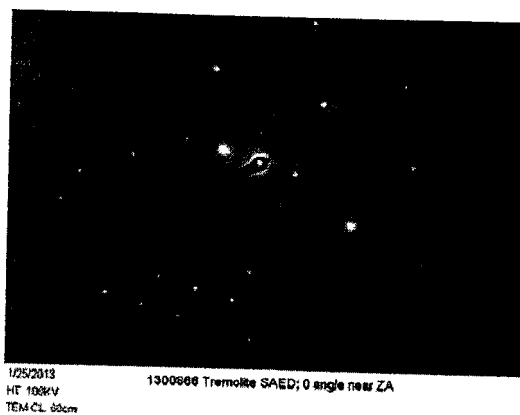
Figure 8: Tremolite asbestos from TEM analysis of releasability air testing of product (images, EDS, and SAED).
