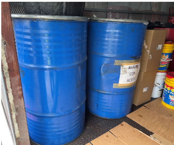
Picture 17- ALCO HIGH TECH PLASTICS — At the Used Oil Storage area, I observed one (1) 55-gallon blue steel drums with impacted rags with used oil not marked with the words, "Used Oil."
