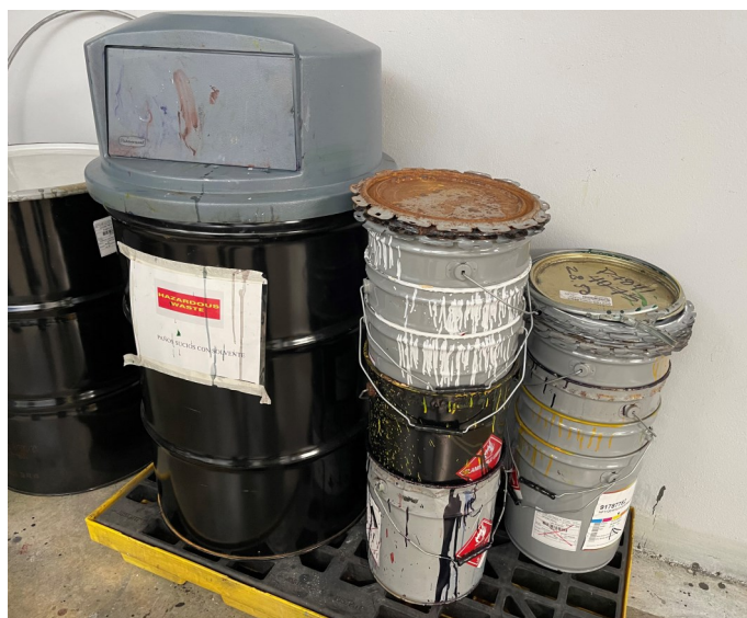
Picture 3 - ALCO HIGH TECH PLASTICS - At the Plastic Extrusion area (SOMA), there was a SSA with (1) 55-gallon black drum with impacted rags with spent liquid solvent waste containing a mixture of propanol and ink, labeled as “Hazardous Waste,” and not identified with its hazard communication pictogram as “Flammable Solids.”
