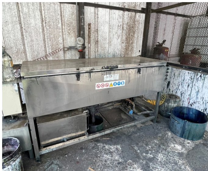
Picture 8 - ALCO HIGH TECH PLASTICS — At the Alcohol Warehouse, I observed a part-washer machine that was used to clean anilox and/or plaster rollers until the new SAA Washing Machine unit was installed nearby the plastic printing machines. This part-washer has been discontinued and emptied over a year ago and is not currently in use.
