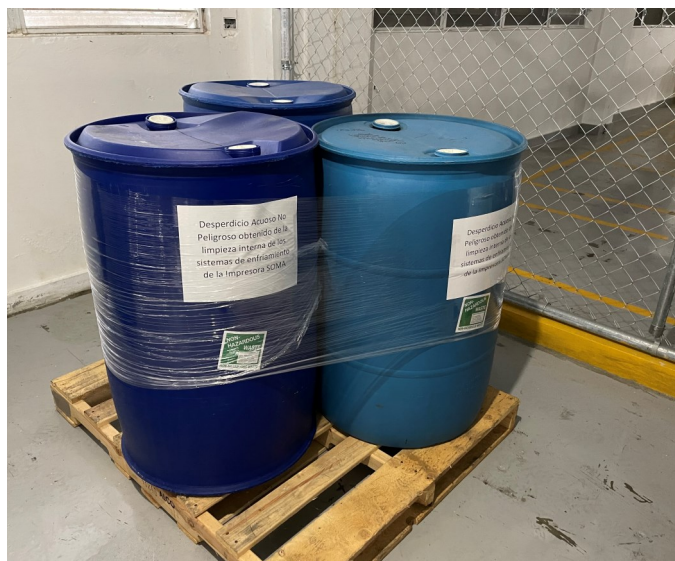
Picture 10 - ALCO HIGH TECH PLASTICS - At the 90-day Hazardous Waste Accumulation area, I observed three (3) 55-gallon blue plastic drums containing aqueous wastes generated from the cleaning activities of the cooling system of the SOMA Printing Machine, all clearly labeled with the words, “Non-Hazardous Waste.”
