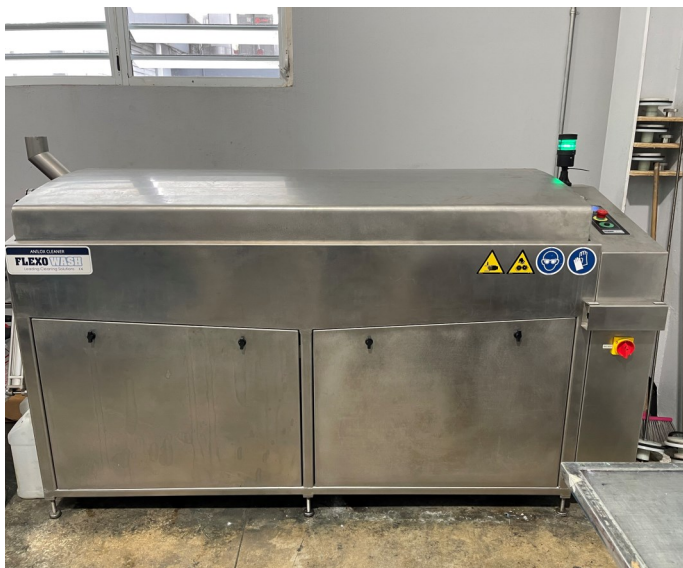
Picture 5 - ALCO HIGH TECH PLASTICS - At the Plastic Extrusion area (SOMA), there was a third SSA with one (1) 300-gallon stainless steel tank used to clean anilox rollers not labeled with the words, “Hazardous Waste,” nor identified with its hazard communication pictogram as “Corrosive Liquids.”
