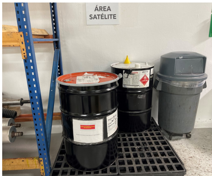
Picture 14 - ALCO HIGH TECH PLASTICS- At the Plastic Lamination one (1) 55-gallon black steel drum with impacted rags contaminated with glue and spent ethyl acetate, labeled as “Hazardous Waste,” and “Paños Sucios con Pega y Acetato,” and was not identified with its hazard communication pictogram as “Flammable Solids”
