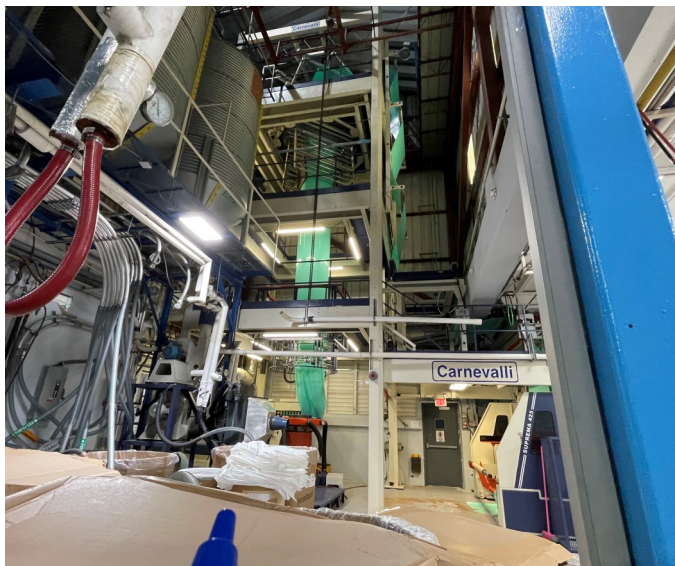
Picture 1 - ALCO HIGH TECH PLASTICS - At the Plastic Extrusion area, a high-volume manufacturing process is undertaken where raw plastic (pellets) is melted and formed into a continuous plastic layer.
