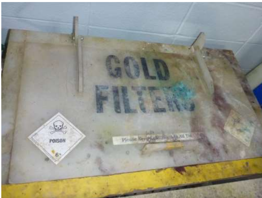
Photo 6: Lid of filter unit to drain filters from the gold plating lines.
