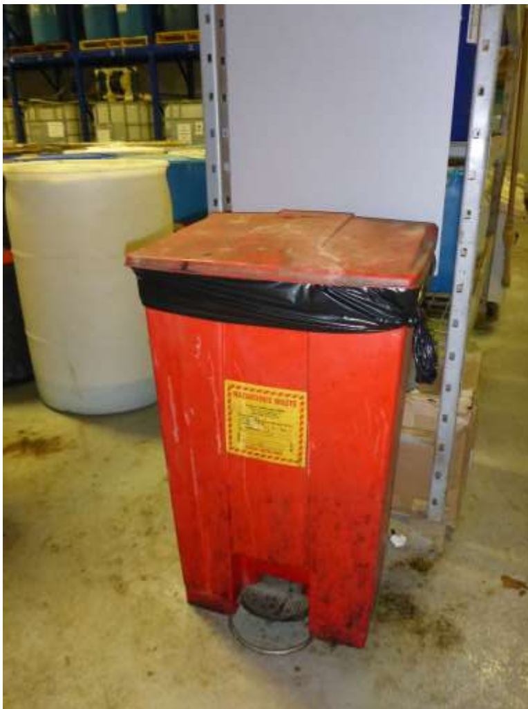
Photo 19: SAA inside the process chemical storage area for accumulating used PPE, absorbents and other solid hazardous wastes.
