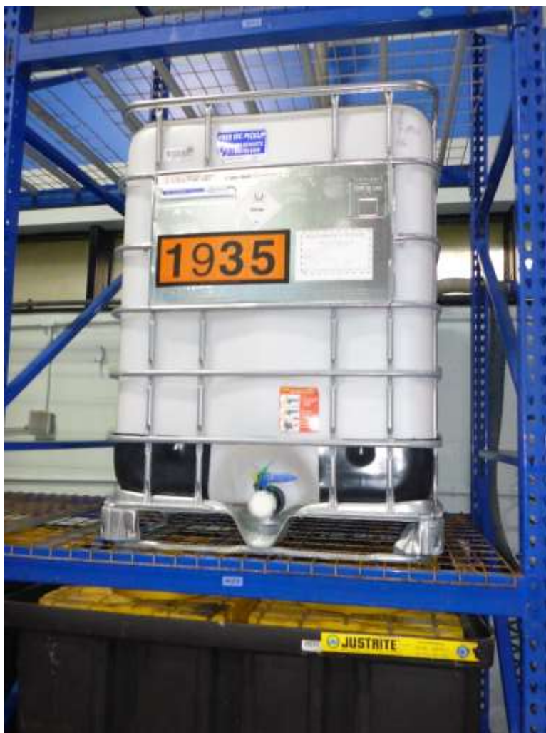
Photo 7: 300-gallon tote labeled F009 / D003 hazardous waste cyanide solution (potassium cyanide) on the middle shelf of the large metal shelving system to the left of the draining units.
