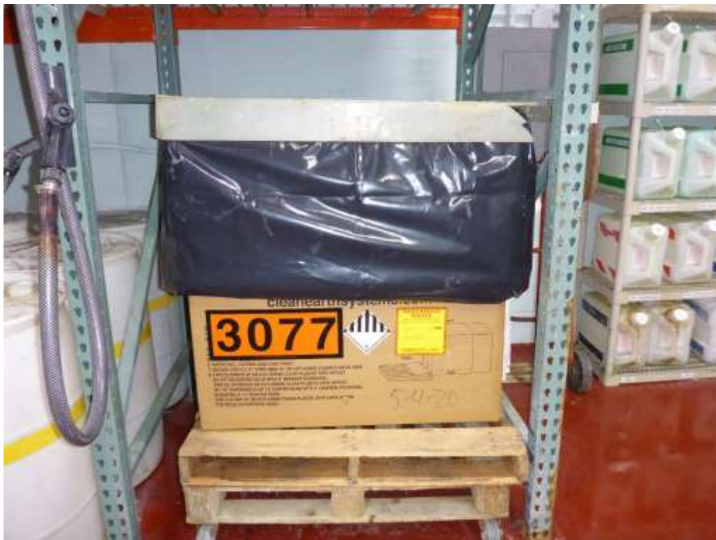
Photo 1: Cubic yard box labeled hazardous waste solid (lead) contaminated filters, PPE, brooms, and floor sweepings on the bottom right shelf of the large metal shelving system in the chemical storage area.
