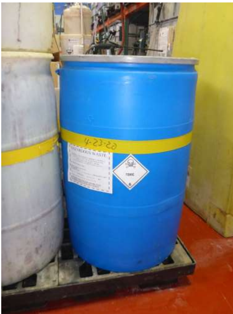
Photo 13: Drum of drained filters from the gold plating line labeled F007 hazardous waste toxic solid inorganic (potassium cyanide) and identified with a toxic hazard placard. The drum was marked with an accumulation start date of 01/23/2020.
