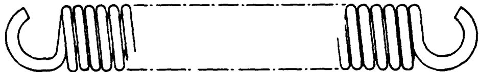
OLD RETURN SPRING 35 COILS WITH IDENTICAL ENDS
