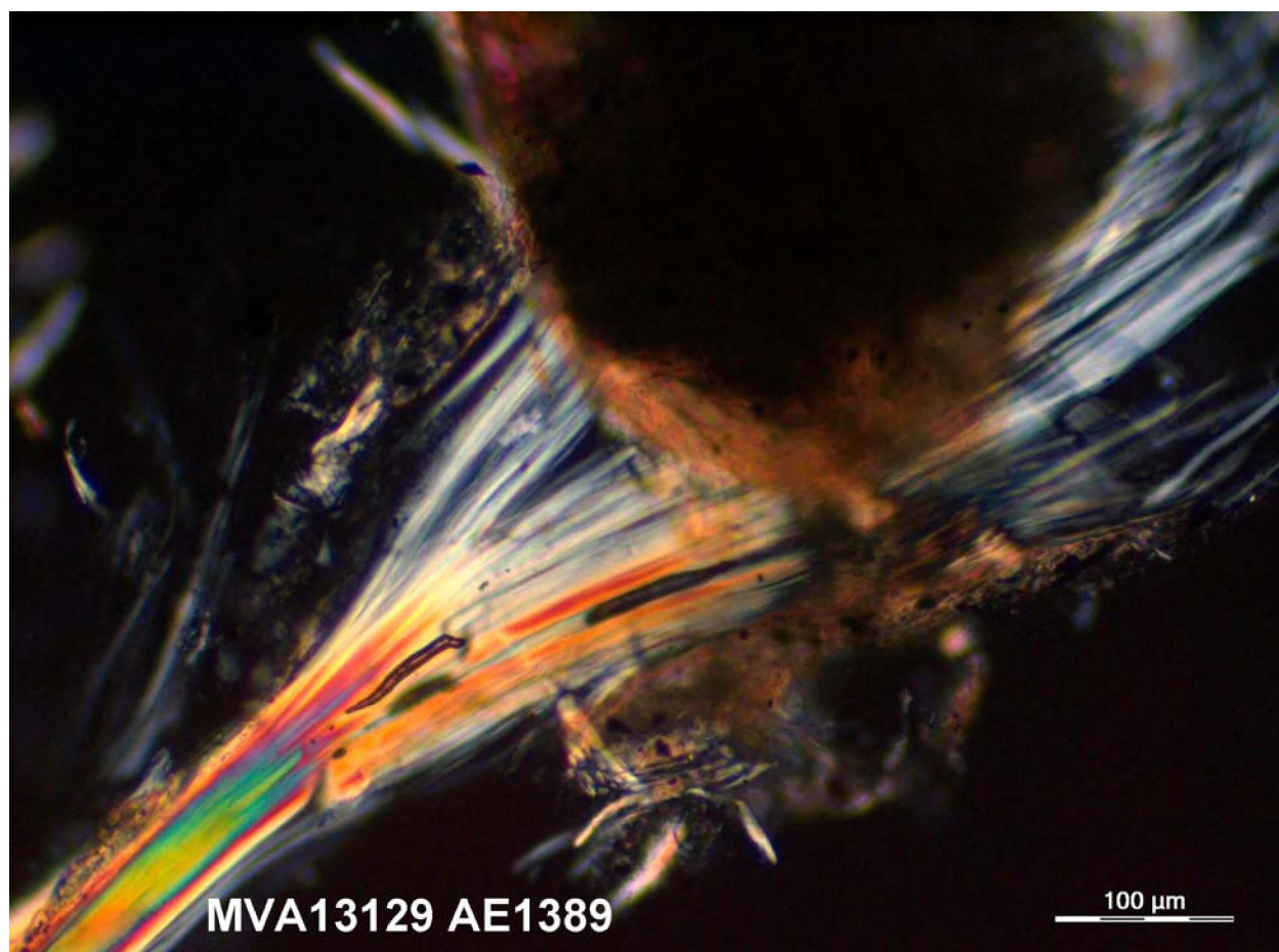
Figure 21. PLM image of chrysotile asbestos fibers and bundles from basewad, sample AE1389.
