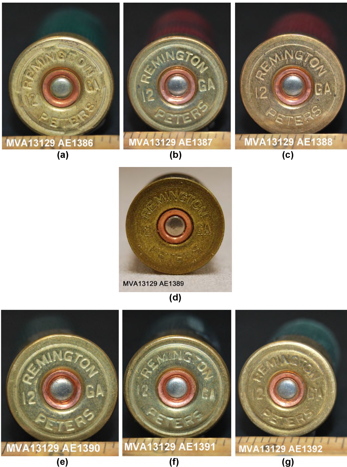
Figure 8. Representative photos of metal base and primer for each style of Remington 12 gauge shotgun shells, samples (a) AE1386, (b) AE1387, (c) AE1388, (d) AE1389, (e) AE1390, (f) AE1391, (g) AE1392. Photograph (d) of AE1389 taken under different lighting conditions. AE1389 metal base appears consistent with other shells when viewed side-by-side.
