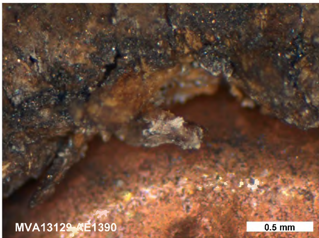
Figure 32. Stereomicroscope image of chrysotile bundle in sample AE1390, after firing.
