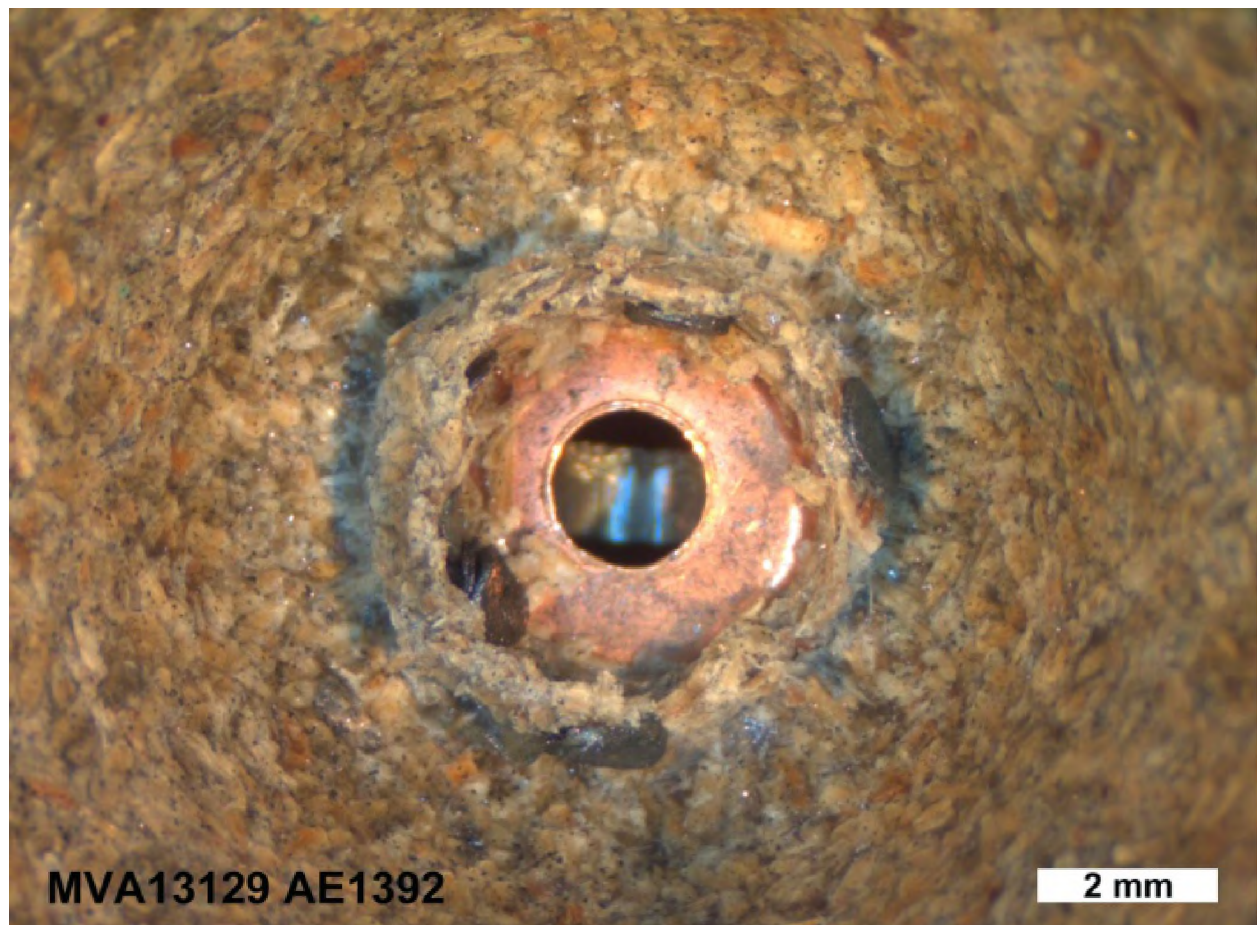
Figure 29. Stereomicroscope image of basewad in sample AE1392.
