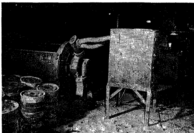
FIG. 6. LOCAL EXHAUST ON TUMBLERS FOR CAST CLEANING.
