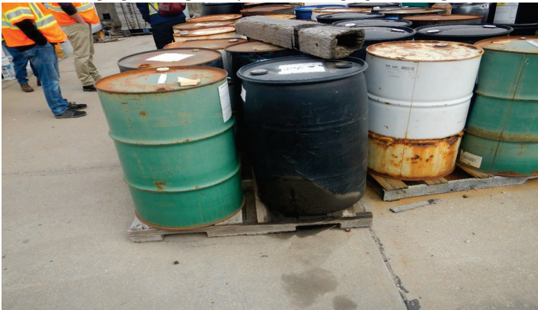
Photo 41, improper storage, leaky drum and improper labeling of drums.
