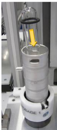
Figure 1: UV lamp quartz housing with FKM O-rings
