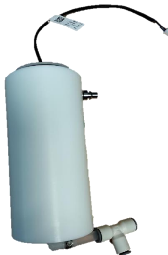
Figure 4: PTFE reactor for UVC light treatment of lab water
