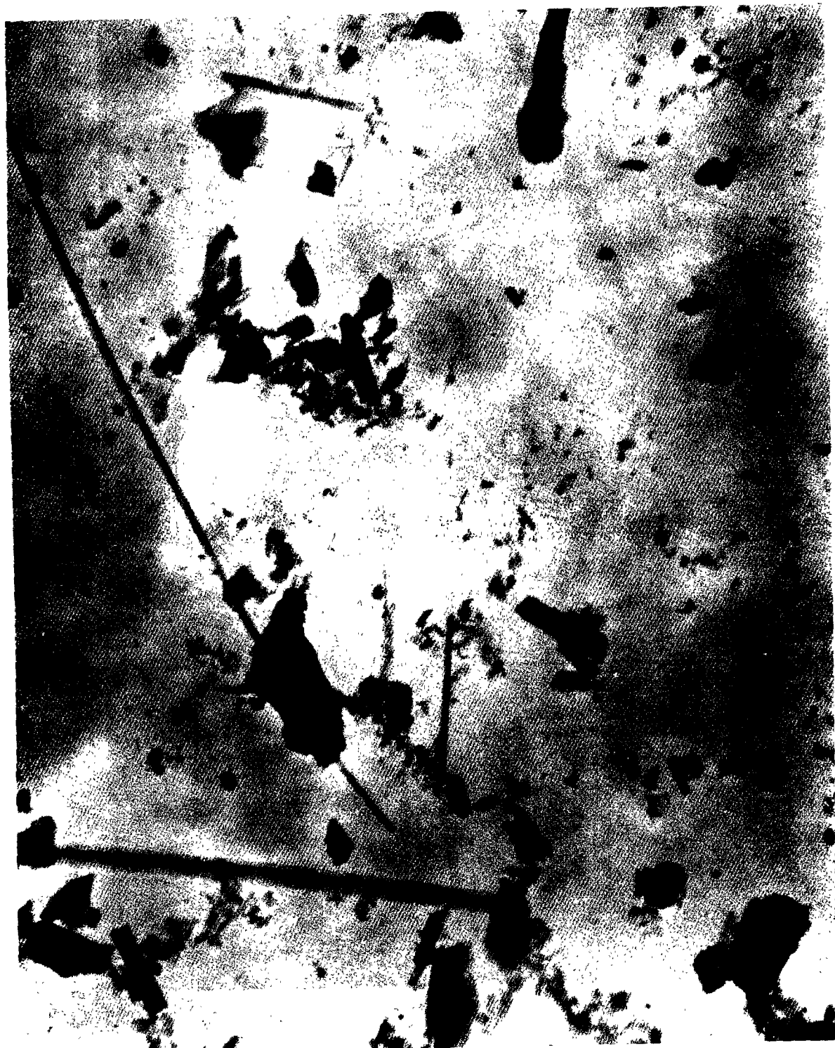
Figure 4. Electron Photomicrograph of Airborne Particulates in Mine and Mill
