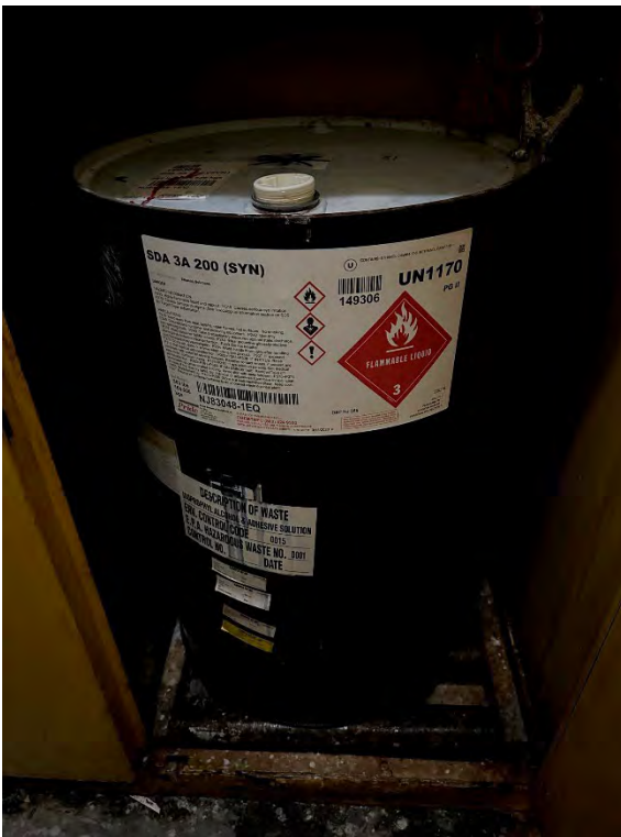
Photograph 4: 55-gallon drum of adhesive and contaminated IPA at the Manufacturing SAA.
