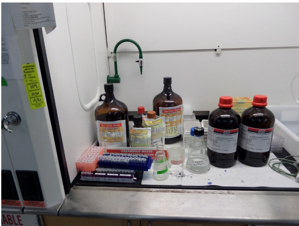
Photograph 7: Hazardous waste containers in a SAA at the biology laboratory section of Room 376 in the Lee T. Todd Building.
