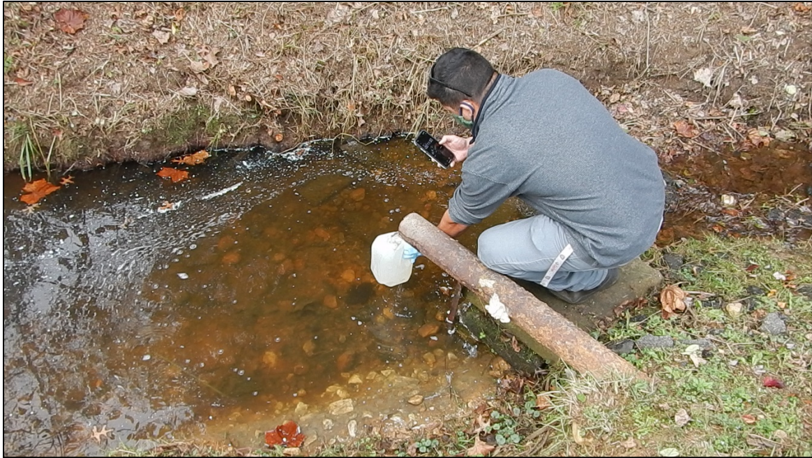
Photograph 17. View of the Plant operator demonstrating how flow is measured at Outfall 001. Flow into a 1-gallon jug is timed once per day. The result is used to calculate gallons per day. Effluent flow was measured at 11.9 seconds per gallon at 10:55 a.m. (approximately 7,200 gallons per day).
