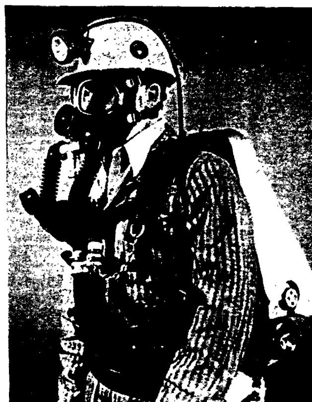
Figure 5-27. Typical oxygen-supplying closed circuit SCBA as used for mine rescue.
