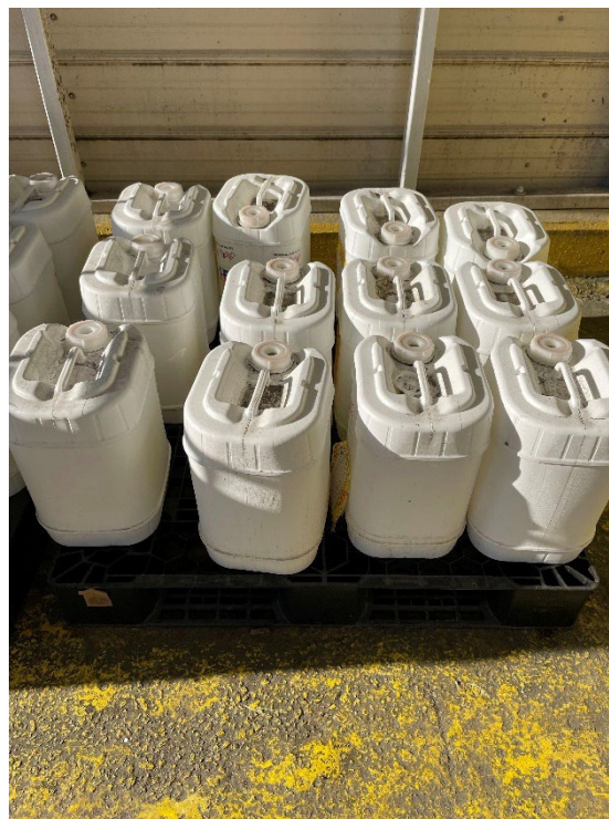
Figure 40: IMG_3283.jpg – Hazardous Waste stored without aisle space
