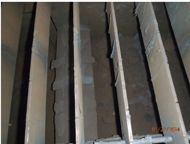
Picture 18 – Fabrication Area burn table with slag
