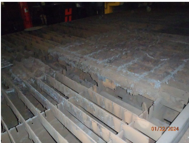
Picture 17 – Fabrication Area burn table with slag
