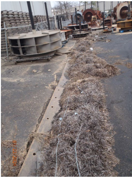
Picture 10 – External Blast Media – non-hazardous black beauty media released to storm water drain
