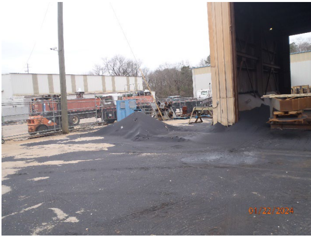
Picture 5 – External Blast Media – non-hazardous black beauty media released to ground
