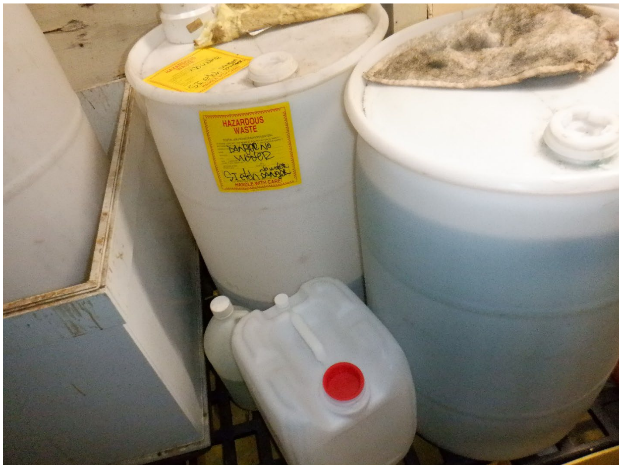
(Figure 10: Showing hazardous waste located in the Central Storage Area with no date and some with no labels)
