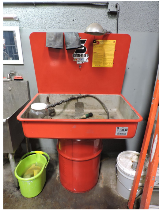
Picture 6— Mechanical Shop Area— At the time of the inspection, a part washer was observed labeled, and dry, but it was open.
