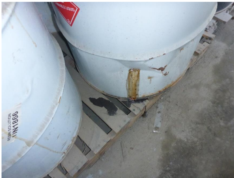
Photo 9: Leaking 55-gallon drum in SA-5. Drum was marked with a flammable liquid DOT hazard placard and appeared to be labeled as hazardous waste. The hazardous waste label could not be read, because it was facing away from the aisle and obscured by other containers.
