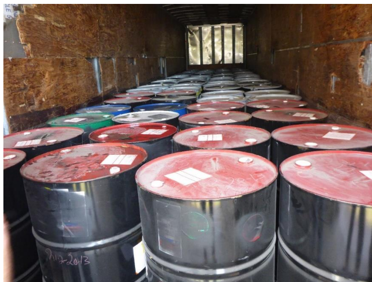
Photo 12: First tractor trailer located at the roll-off container CAA. The trailer is full of 55-gallon drums, which were full of hazardous waste generated off-site and received by the facility for treatment, storage and / or disposal.
