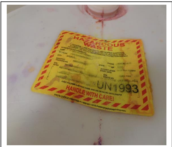
Atlanta VA. Clinical Laboratory Room 2B-176 90-Day Area. The inspectors observed the label on the container appeared to be deteriorating. Photograph 11 taken at 11:16 a.m.
