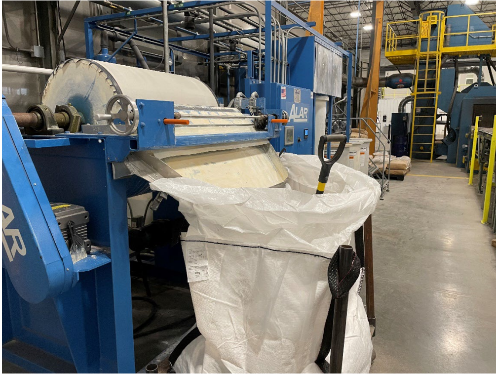
Photo #5. Accumulated solids from the vacuum filtration unit are collected in the tote bag.
