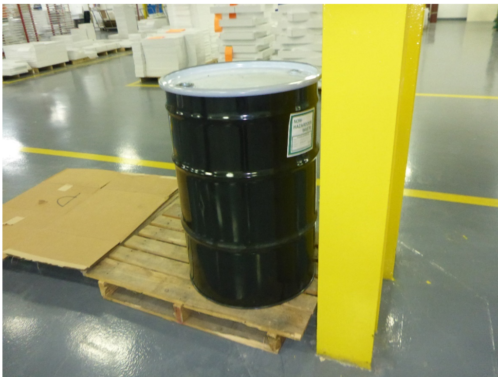
Photo 17: One 55-gallon drum of excluded solvent contaminated disposable wipes observed near the end of the first solvent paint spray line. The drum was closed and labeled non-hazardous solvent excluded rags.
