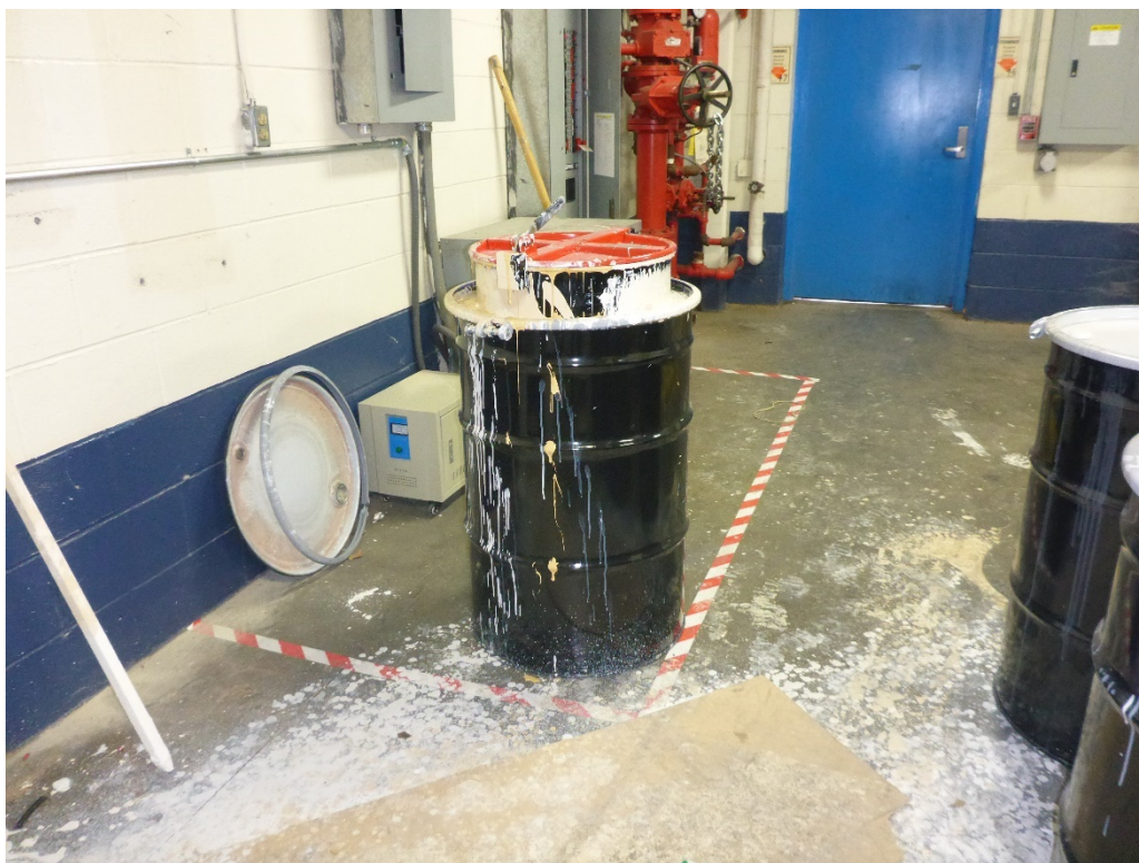
Photo 6: One 55-gallon drum observed near the wall near the solvent distillation unit in the Reclaim Room. According to facility personnel, solvent sludge generated in the distillation unit is manually transferred into this drum using a 5-gallon bucket. The drum is fitted with an elevated lid, which was latched closed. The drum was not labeled as “hazardous waste,” it was not marked with an accumulation start date, and it was not marked with an indication of the hazards of its contents.
