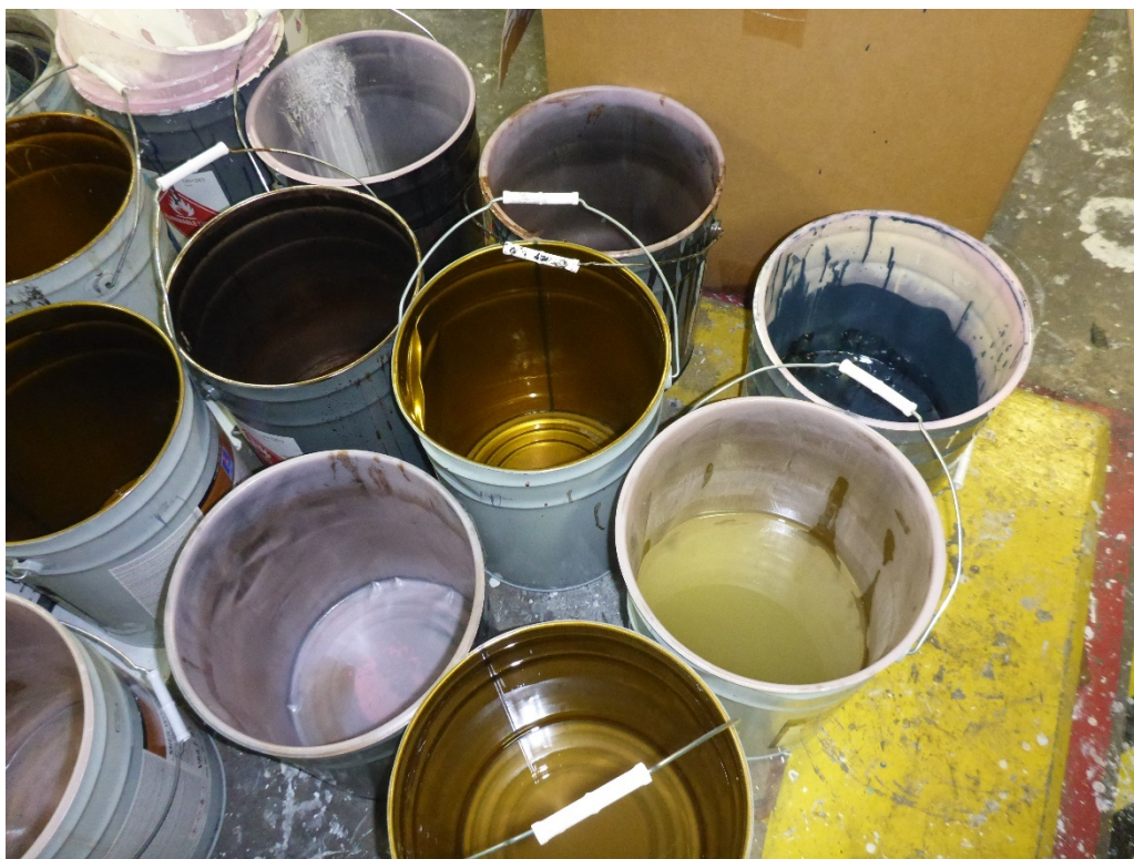
Photo 11: Several of the 5-gallon buckets in the Reclaim Room. Buckets appear to contain spent solvents and/or solvent paint waste. The buckets are open and not labeled.
