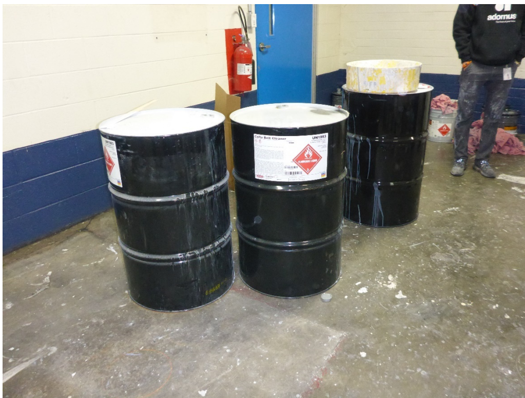
Photo 8: Three 55-gallon drums observed in the Reclaim Room near the wall opposite the solvent distillation unit. According to facility personnel, two of the drums contain new or recovered Cefla Belt Cleaner solvents, and the third drum, which is equipped with an open funnel, is used to accumulate reclaimed Cefla Belt Cleaner solvent that is generated in the solvent distillation unit in this room.
