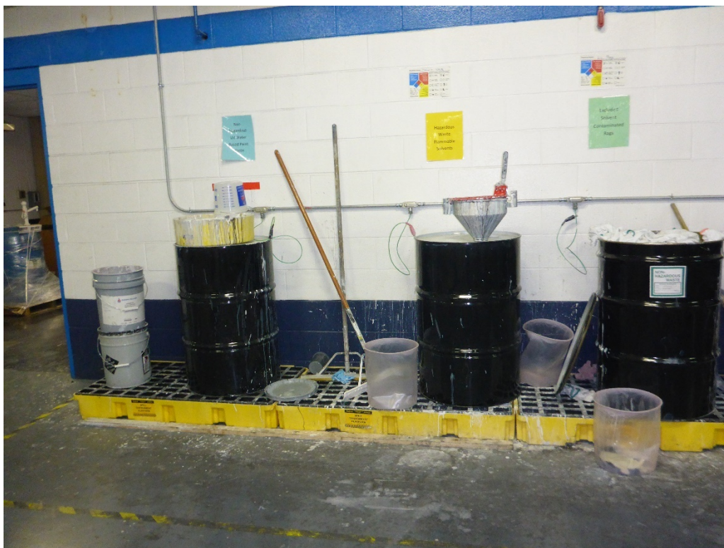
Photo 1: Three of five 55-gallon drums staged on portable secondary containment pallets in the UV Paint Coating Area along the wall just outside of the Paint Mixing Room. The drum on the left was identified for accumulating nonhazardous UV water based paint; the drum in the middle was identified for accumulating hazardous waste flammable solvents; and the drum on the right was identified for accumulating excluded solvent contaminated disposable wipes.
