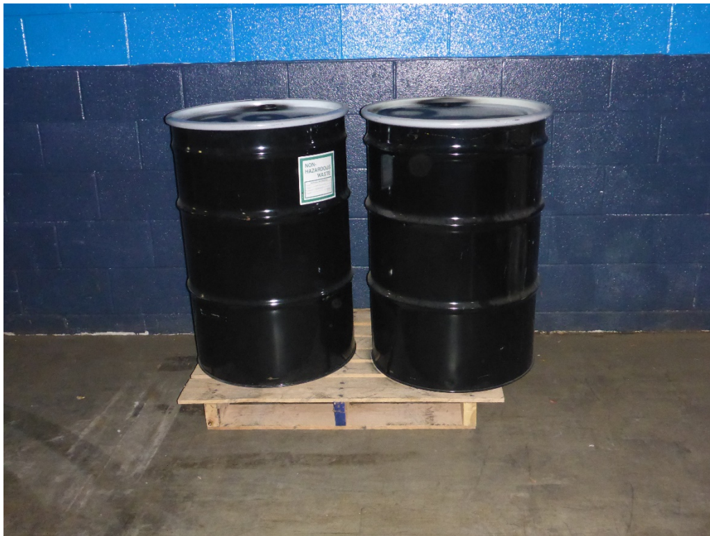
Photo 25: Two 55-gallon drums of excluded solvent contaminated disposable wipes observed in the hazardous waste CAA. The drums were both closed and labeled nonhazardous excluded solvent contaminated rags.
