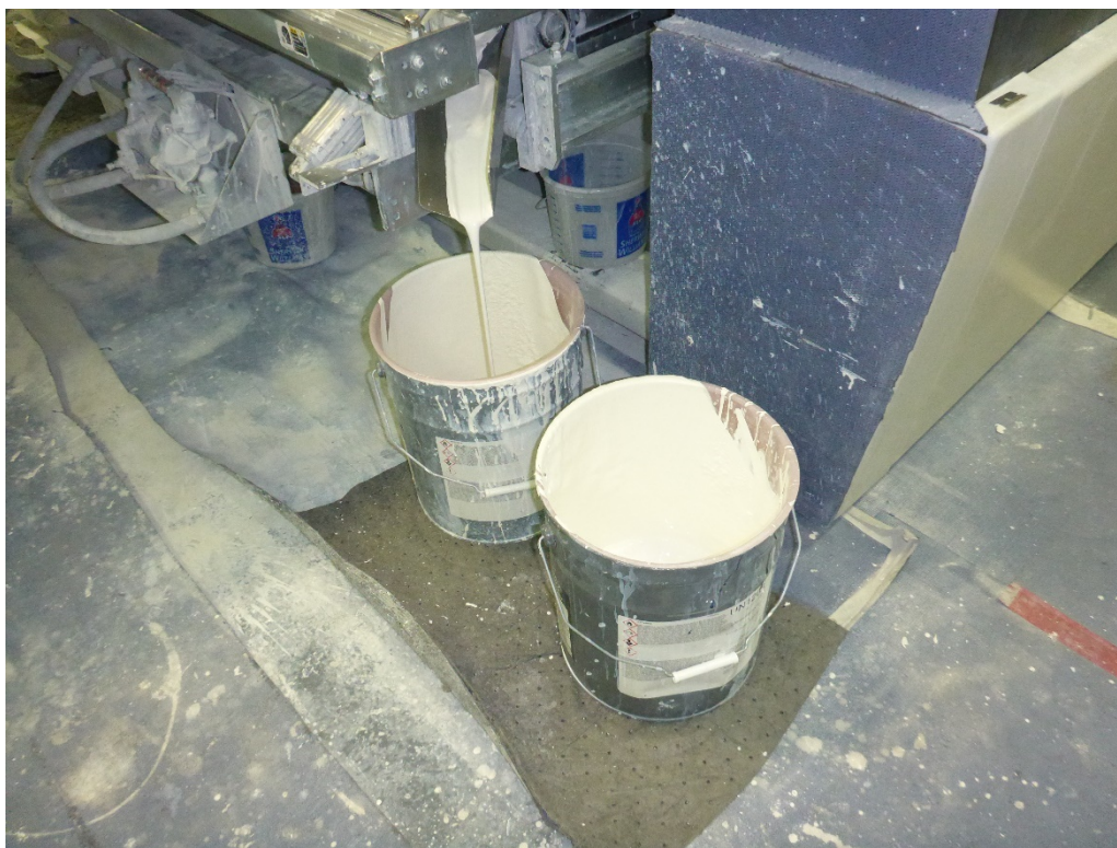
Photo 13: Two 5-gallon buckets staged at the first solvent paint spray line SAA. These buckets are used to accumulate D001 / F003 / F005 hazardous waste flammable liquid (toluene / acetone) that is generated as excess paint and overspray in this solvent paint spray line unit. Neither bucket is labeled with the words “hazardous waste.” Neither bucket is closed, but only one has waste being added into the container.
