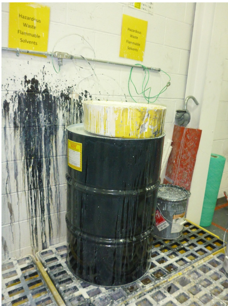
Photo 15: One 55-gallon drum located in the first solvent paint spray line SAA. The drum is located on a secondary containment pallet next to the process line. D001 / F003 / F005 hazardous waste flammable liquid (toluene / acetone) that is generated as excess paint and overspray in the solvent paint spray line is poured from the 5-gallon buckets staged at the spray line into this 55-gallon drum. The drum is equipped with an open funnel. It is labeled as D001 / F003 / F005 hazardous waste flammable liquid (toluene / acetone) and it is identified with a flammable liquid DOT hazard placard.
