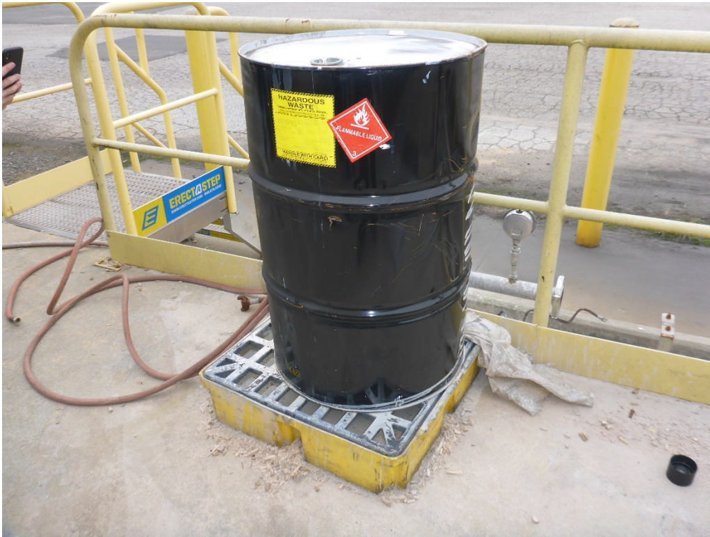
Photo 26: One drum of hazardous waste observed on a secondary containment pallet on the loading dock outside of the hazardous waste CAA. The drum was labeled D001 / F003 / F005 hazardous waste flammable liquid (acetone / toluene) and identified with a flammable liquid DOT hazard placard. The drum was dated 10/07/2020, and the secondary containment unit was full of liquid. Mr. Lucas explained that the drum was hit with a forklift during loading activities, which caused it to leak. Because the leaking drum could not be loaded onto the truck for transport off-site, it was moved out to this portable secondary containment unit
