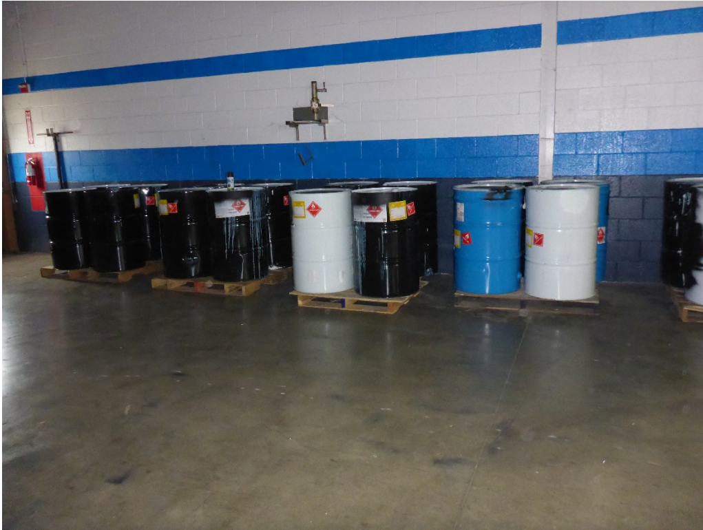
Photo 22: Twenty 55-gallon drums of hazardous waste observed in the hazardous waste CAA. The drums were staged on six wooden pallets. Hazardous waste labels were observed on seventeen of the drums, indicating that the containers held D001 / F003 / F005 hazardous waste flammable liquids (acetone / toluene). Hazardous waste labels were observed on the remaining three drums, but the labels were obscured by other drums or the wall and could not be read. No accumulation start dates were observed on three drums. The oldest drum with an accumulation start date was dated 02/05/2021. Although all of the drums were identified with a flammable liquid DOT hazard placard, that placard had been partially covered with black spray paint on two of the drums.
