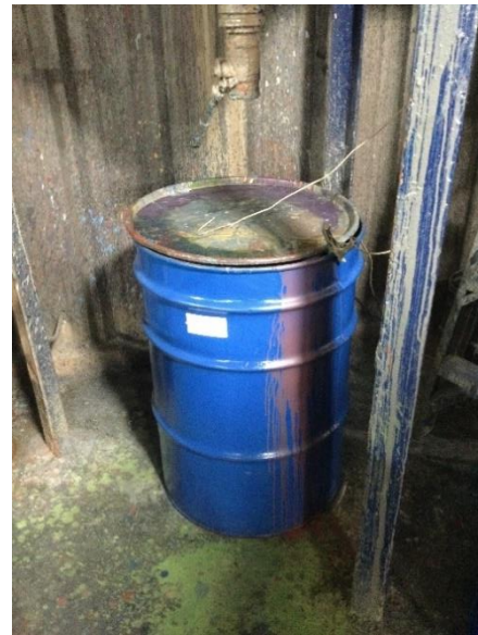
Photo 12: One (1) 55-gallon container of sludge waste with no hazardous waste label, no hazard indication, and open.
