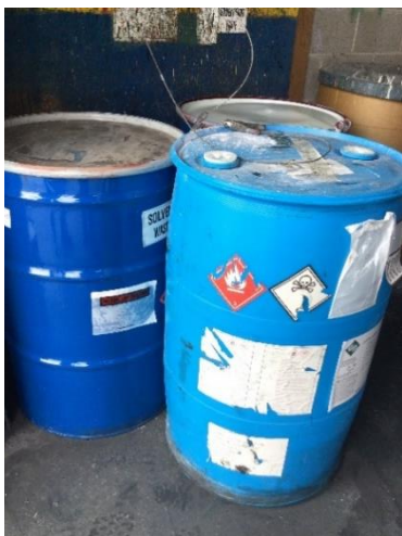
Photo 17: One (1) 55-gallon container of highly concentrated solvent waste, no hazardous waste label, and a hazard indication.
