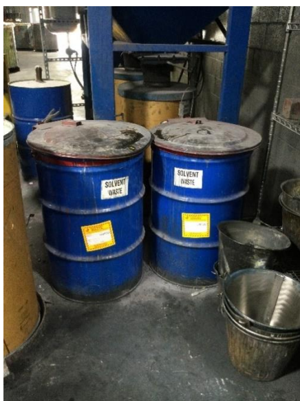
Photo 25: The inspectors also observed two (2) 55-gallon containers of solvent waste, labeled “hazardous waste”, not properly closed, and not marked with a hazard identification.
