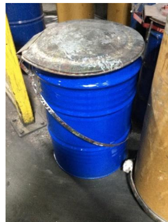
Photo 24: One (1) 55-gallon container of solvent-contaminated wipes. The container was not properly closed and was missing a label and did not have an accumulation start date.
