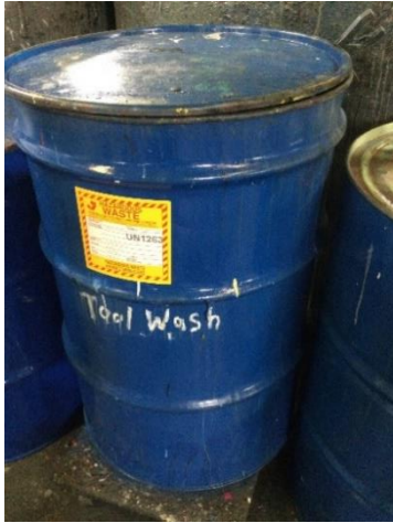
Photo 29: One (1) 55-gallon container of tool wash, labeled “Hazardous Waste”, not marked with an indication of hazard, and the container was open.
