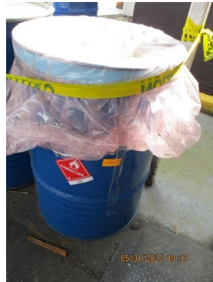
Photo 4: 55-gallon container of solvent waste, open, no hazardous waste label or start accumulation date.
