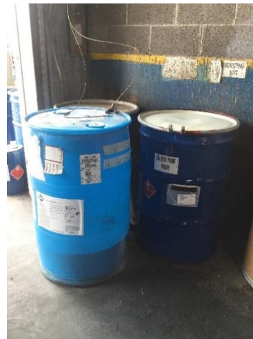
Photo 16: One (1) 55-gallon container of solvent paint-mixed solids, closed, with a small hazardous waste label and an indication of hazard.
