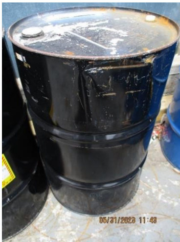
Photo 31: 55-gallon container in CAA with no label, hazard identification, or start accumulation date.
