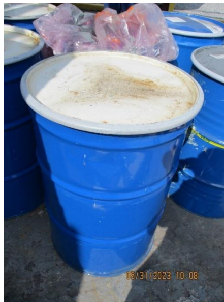
Photo 6: 55-gallon container of solvent waste. No hazardous waste label, no start accumulation date.
