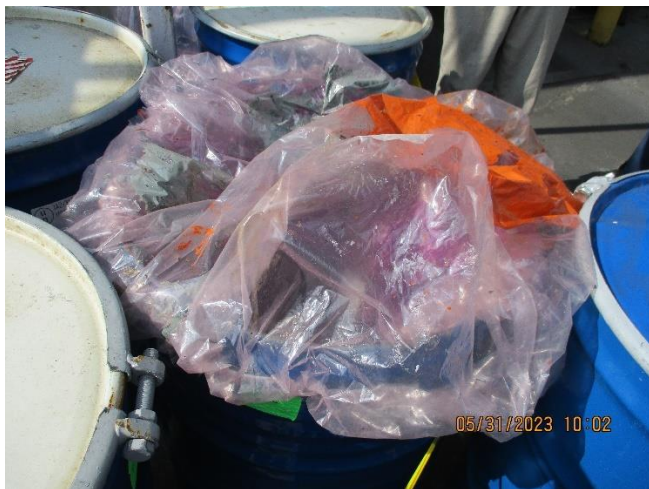
Photo 7: 55-gallon container of solvent waste, open, no hazardous waste label, no start accumulation date.
