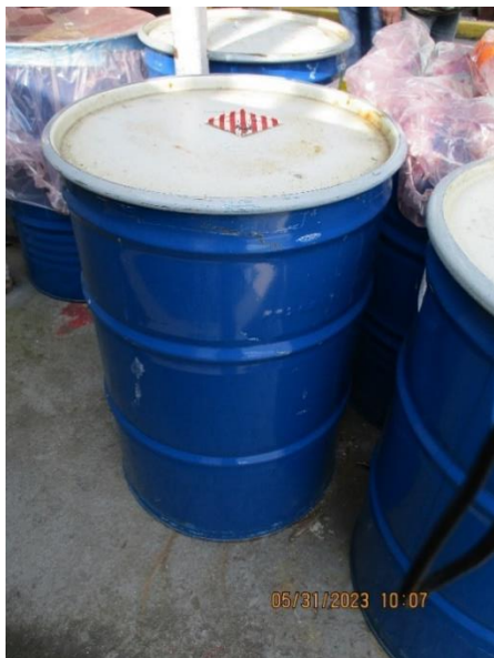
Photo 5: 55-gallon container of pigment waste. No hazardous waste label, no start accumulation date.
