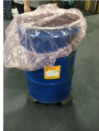
Photo 22: One (1) 55-gallon container of solvent waste. The container was open with just a plastic cover, labeled “Hazardous Waste”, and missing a hazard indication
