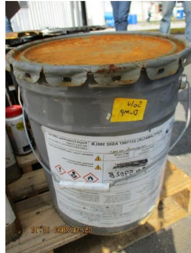
Photo 10: 5-gallon container that did not have a secure lid and containing solvent-based primer material inside.
