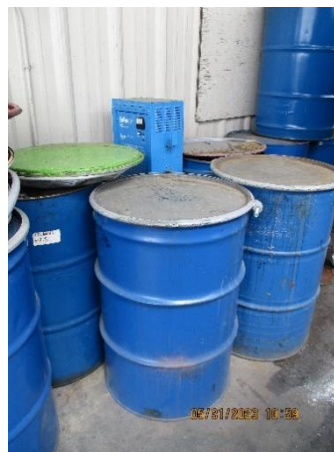
Photo 20: Two (2) 55-gallon containers that appeared to have material inside and did not have any sort of labeling (photo).
