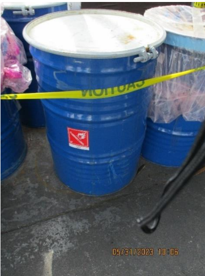
Photo 3: 55-gallon container of pigment waste. No hazardous waste label, no start accumulation date.
