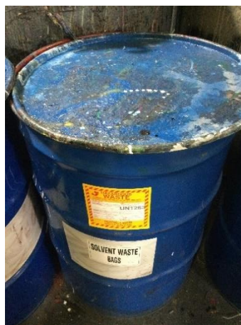
Photo 28: One (1) 55-gallon container of solvent waste bags, labeled “Hazardous Waste”, not marked with an indication of hazard, and the container was open.
