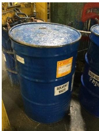
Photo 27: One (1) 55-gallon container of solvent waste, labeled “Hazardous Waste”, not marked with an indication of hazard, and the container was open.
