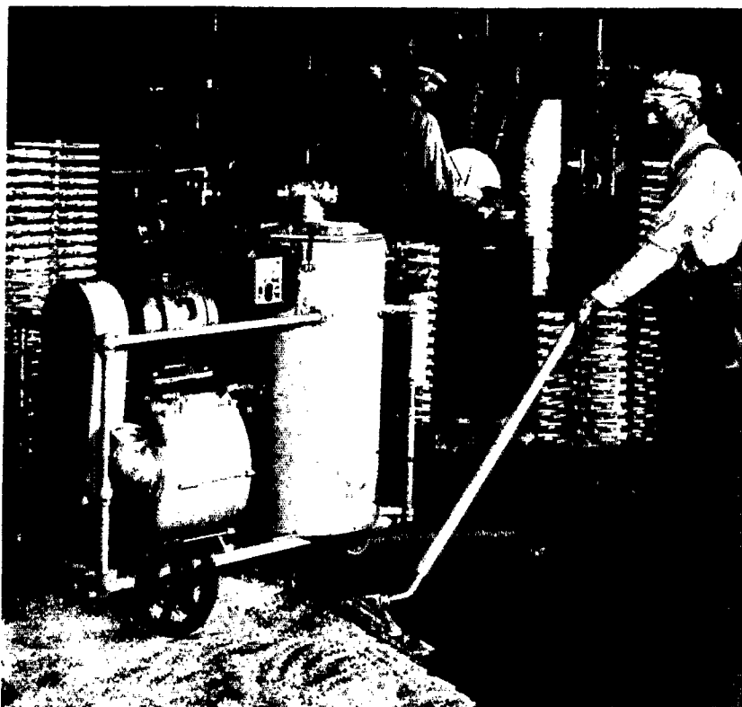
Dust is not raised when floors are cleaned by suction.
