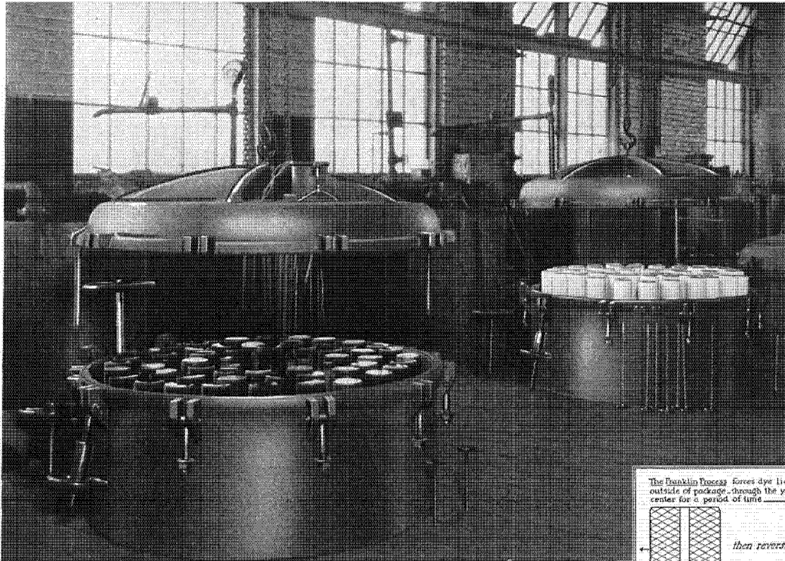
Left—Franklin Process machines loaded, before and after dyeing
