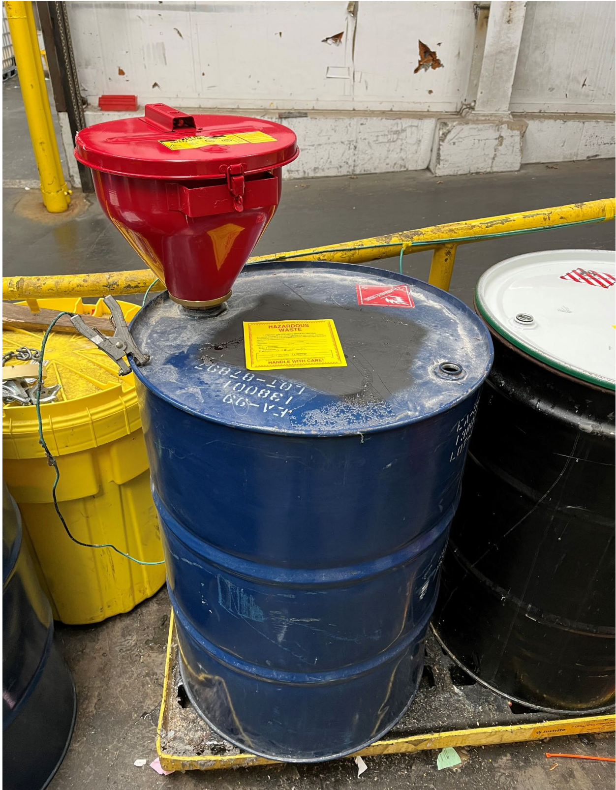
Photo #1: View of the container of hazardous waste with the screw cap missing.
