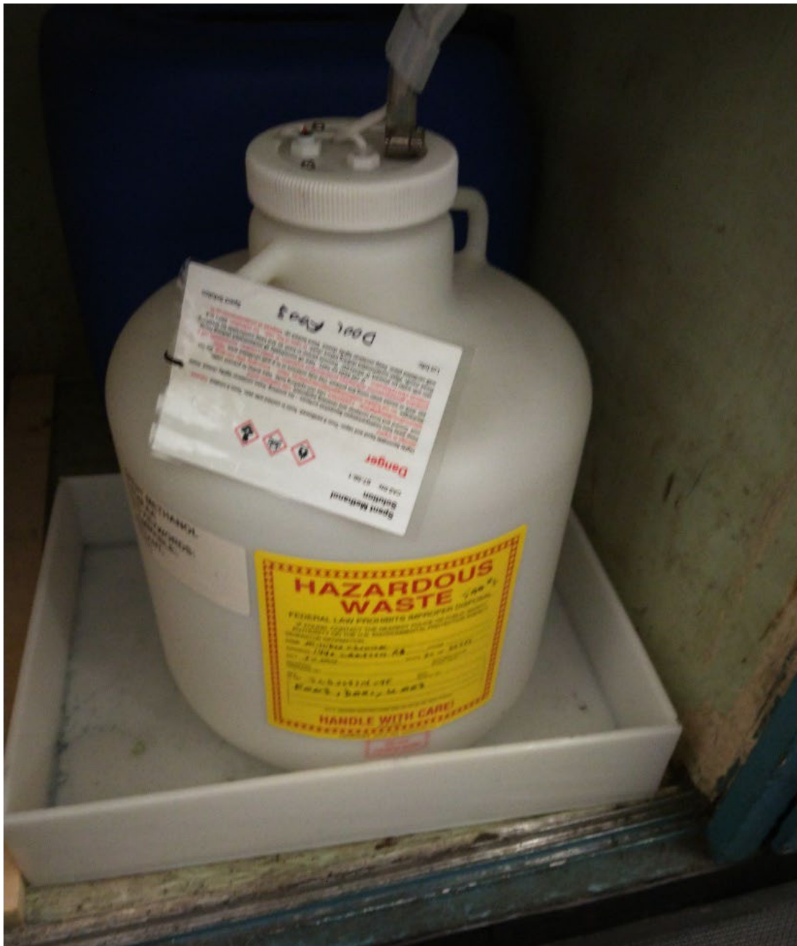
Photograph 3: SAA 2 with 5-gallon container connected to the AA unit with a hose collecting spent methanol from atomic absorption unit - D001, F003, U003
