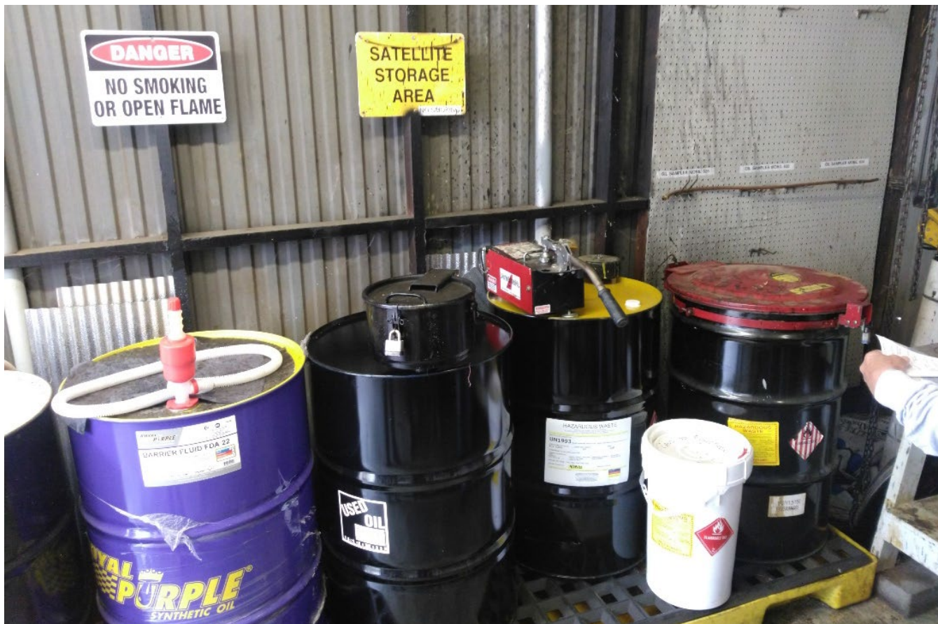
Photograph 1: Maintenance Warehouse Oil Shed: 5-gallon with aerosol cans and one 55-gallon container with an aerosol can puncturer, one 55-gallon used oil container and one 55-gallon container of solvent contaminated shop rags.
