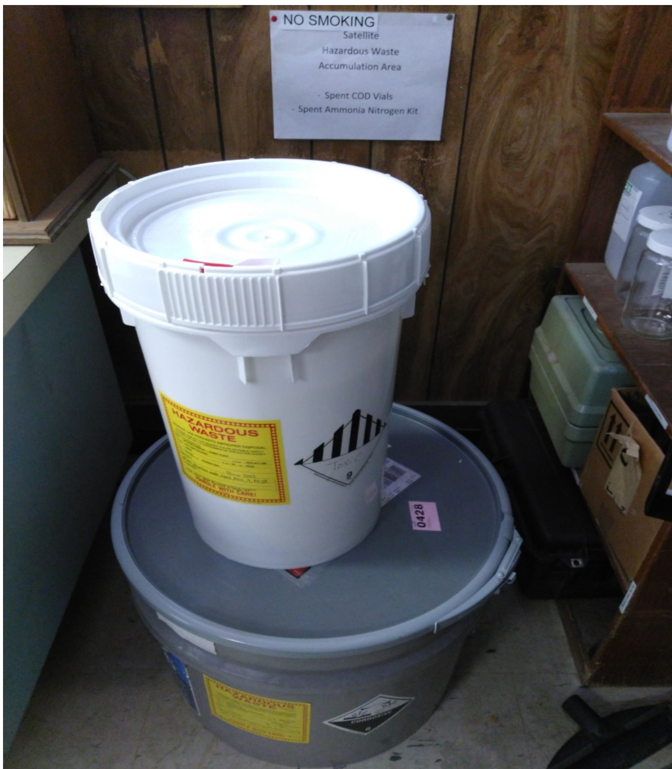
Photograph 10: Hazardous waste containers in the wastewater laboratory's SAA.
